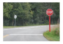
The cost to install reflective tape on existing stop sign poles is estimated to be up to \$200 per pole, while the cost for installation of reflective panels on post is up to \$350 per pole. Tape is highly reflective, with an effective life span of 3 to 10 years. Reflective panels last around 7 years.
