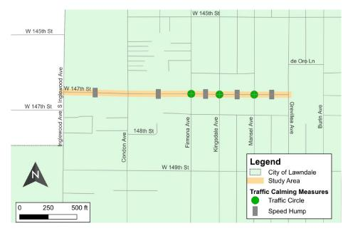
The incorporation of the traffic circles and speed humps will include signage, pavement markings and minor stripping changes.
