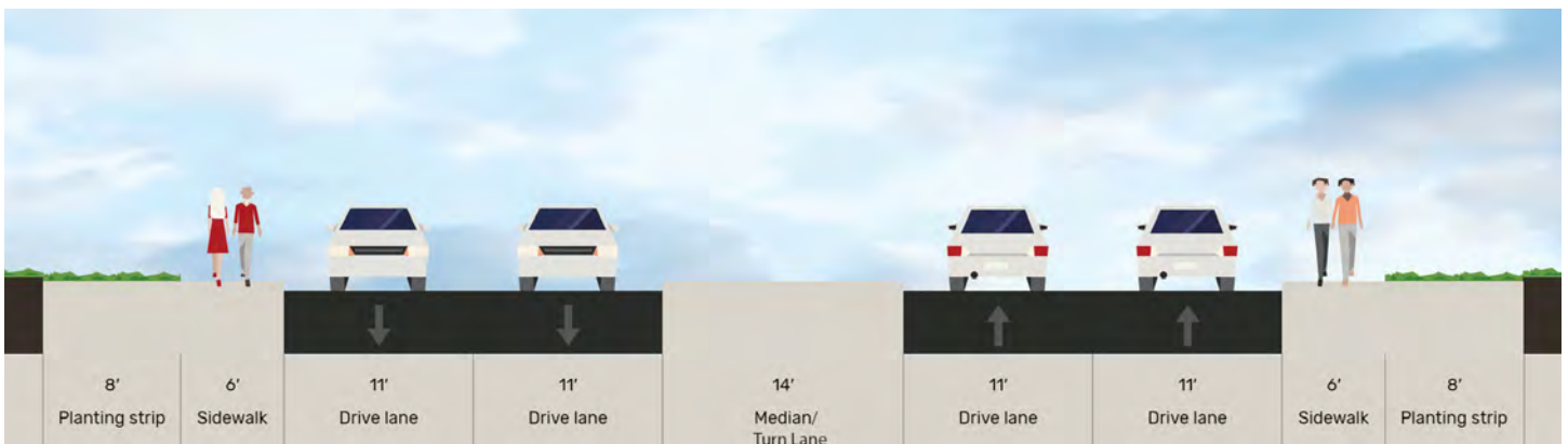
Figure 4.8 | Minor Arterial - 4 lanes, divided
