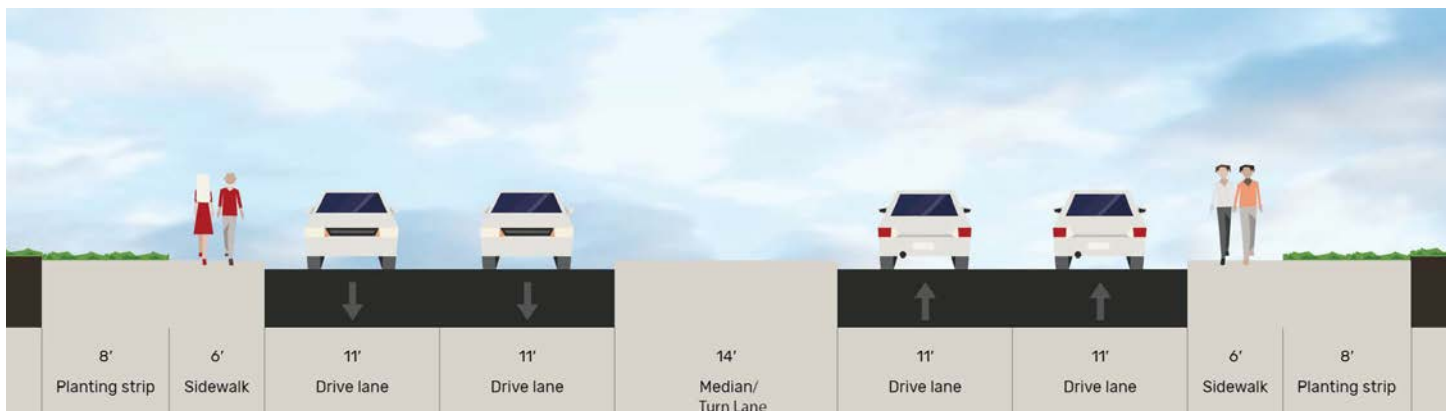
Figure 4.8 | Minor Arterial - 4 lanes, divided
