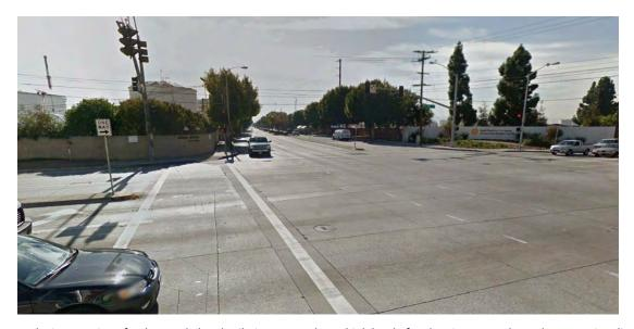
The intersection of Del Amo Blvd and Wilmington Ave has a high level of pedestrian stress due to long crossing distances, high speeds, and multiple travel lanes.
