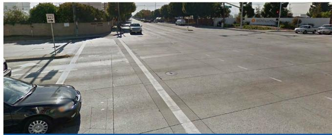
The intersection of Del Amo Boulevard and Wilmington Avenue has a high level of pedestrian stress due to long crossing distances, high speeds, and multiple travel lanes.
