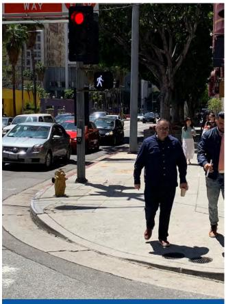
LPIs provide pedestrians with a head start into an intersection before vehicles are given a green phase.
