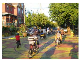
Bicycle boulevards are established on streets that improve connectivity to key destinations and provide a direct, low-stress route for bicyclists, with low motorized traffic volumes and speeds, designated and designed to give bicycle travel priority over other modes.
