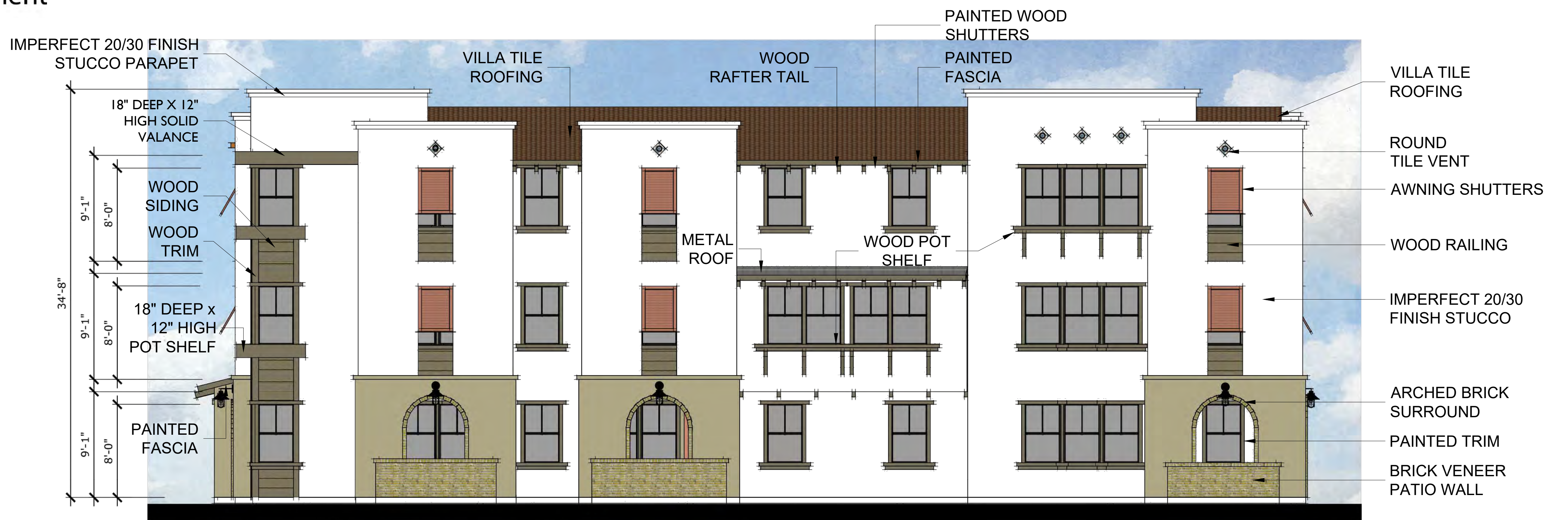
BLDG 1 - FRONT ELEVATION
