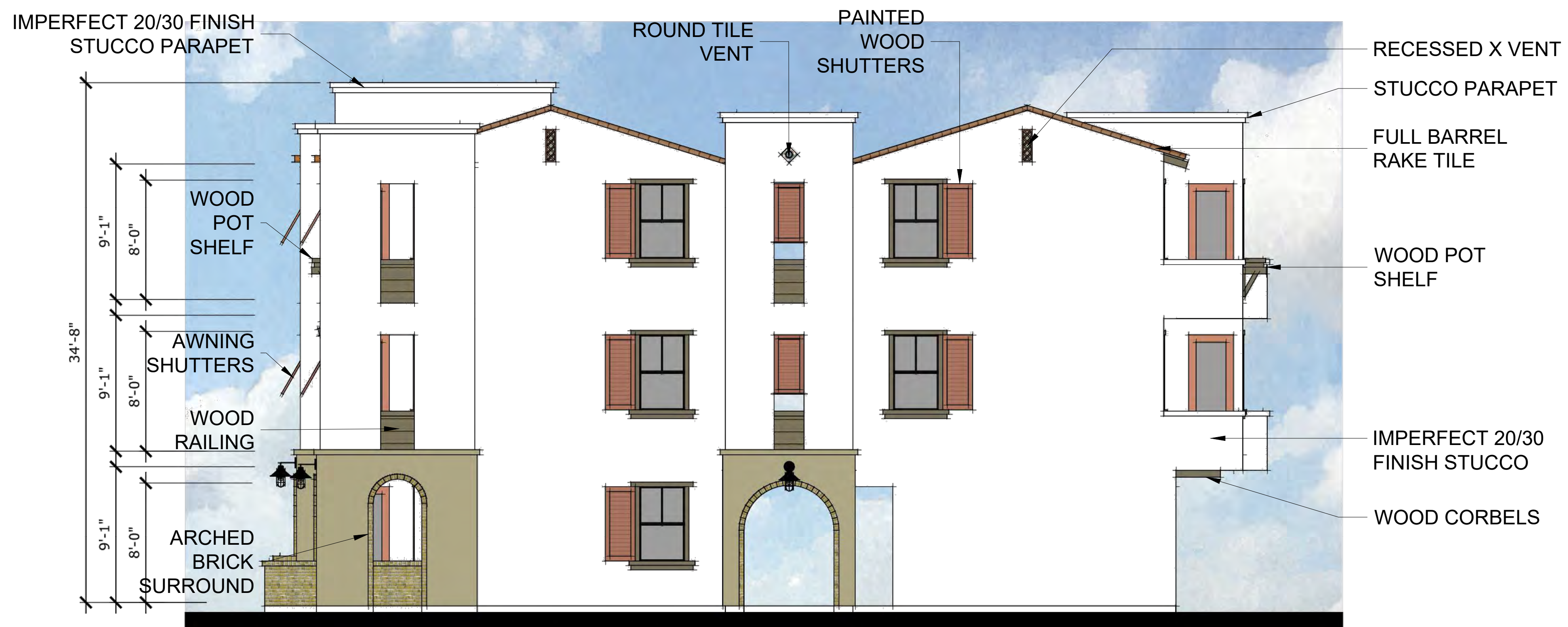
BLDG 1 - RIGHT ELEVATION
