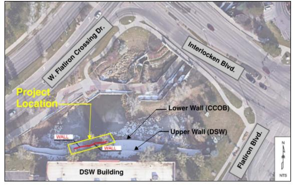
The lower wall and the upper wall are stabilizing a very steep grade. The lower wall is on CCOB property and a section of the wall is failing. This portion of the wall is sagging and showing other signs of distress such as improper drainage. The integrity of this retaining wall is crucial in supporting the above property, 595 Flatiron Boulevard, formerly the DSW retail store. This proposed work will make the necessary repairs in order to prevent a major failure of the lower retaining wall.
