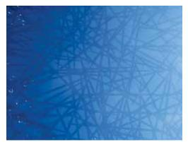
Ornilux Mikado's pattern reflects UV wavelengths. The spiderweb effect is visible only from very limited viewing angles. Photo courtesy of Arnold Glass
