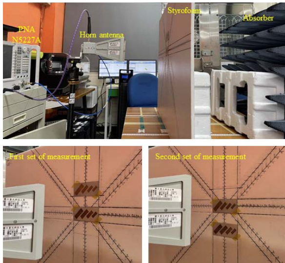
Fig. 10. Photographs of the experiment for separating mixture backscattering signals.
