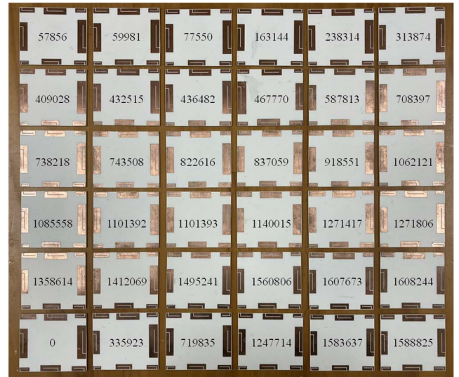
FIGURE 16. Photograph of the test pieces of chipless tags.
