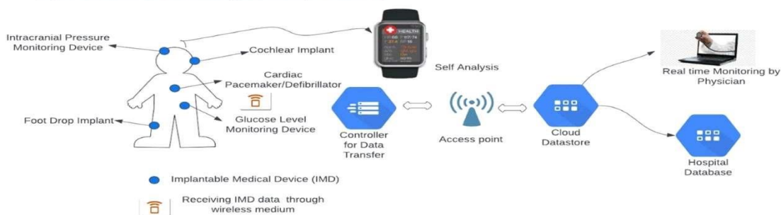
Model of an implantable medical device with biotelemetry [17]
