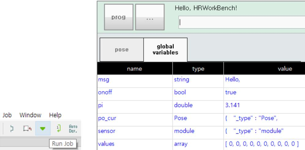
The screenshot shows a software interface with a 'Run Job' button in the bottom left. The main window displays a table of global variables. The table has columns for 'name', 'type', and 'value'. The variables listed are: msg (string, Hello), onoff (bool, true), pi (double, 3.141), po\_cur (Pose, { "\_type": "Pose", ...}), sensor (module, { "\_type": "module", ...}), and values (array, [ 0, 0, 0, 0, 0, 0, 0, 0, 0, 0 ]).
