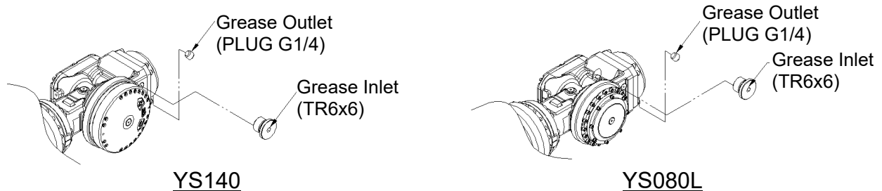
Figure 5.7 R1-Axis Reducer Grease Inlet/Outlet
