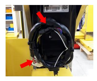
(3) Disconnect the Z-axis connector and cable.
