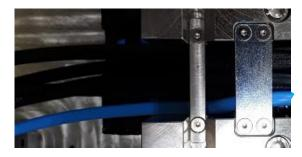
(6) Remvoe the cable fixing plate from the x-axis carriage and remove the cable and cableveyor from the x-axis base.
