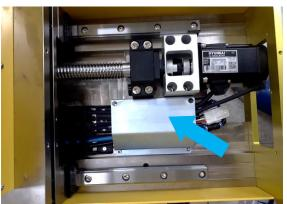
(3) Disconnect the Z-axis connector and cable.
