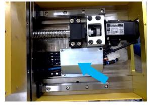
(4) Remove the connector cover from the Y-axis base.
