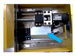
(3) Remove the connector cover from the Y-axis base.
