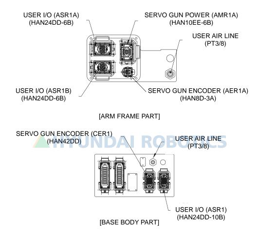
Figure 2.8 Application Wiring and Inspection Wiring Diagram: [HH130L/HH200]
