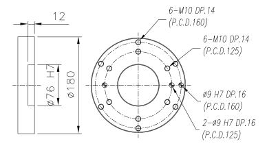
Figure 2.6 Details of Wrist Axis Attachment Surface: [HH130L/HH200]
