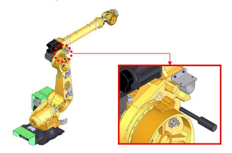
Figure 6.2 2<sup>nd</sup> Arm (V-axis) Fixing Pin Insertion Position
