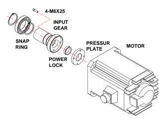
Figure 6.3 Axis S motor assembly
