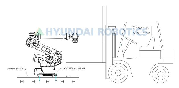
Figure 3.4 How to Transport : Using forklift [HH130L/HH200]
