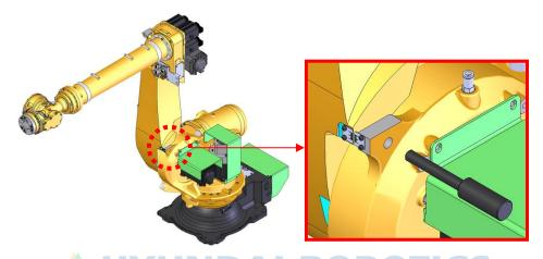
Figure 6.1 1st Arm (H-axis) Fixing Pin Insertion Position
