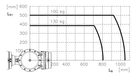
Figure 3.7 Wrist Axis Torque Mapping: [HH130L]
