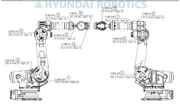
Figure 4.1 Inspection Part for Main Bolts [HH130L]
