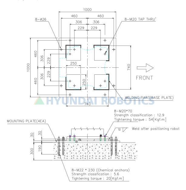
Figure 3.6 Dimension of Robot Installation: [HH130L/HH200]
