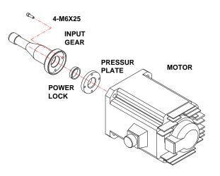
Figure 6.4 Axis H&V Motor Assembly
