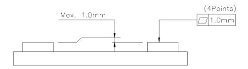
Figure 3.5 Accuracy of Installation surface
