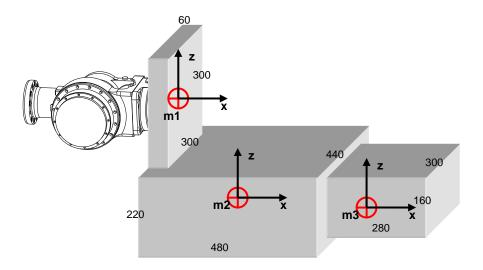
Figure 3.11 3-D load model 3-D shape
