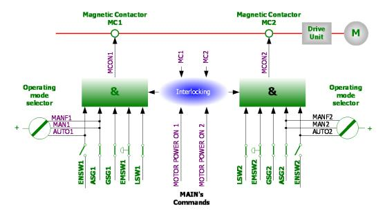
Figure 1.5 Configuration for safety chain
