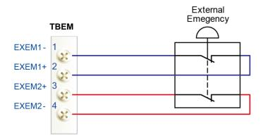
Figure 1.6 Connection with external emergency halt switch through system board terminal block TBEM
