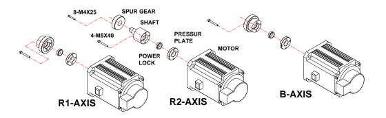
Figure 6.5 Wrist Axis Motor Assembly
