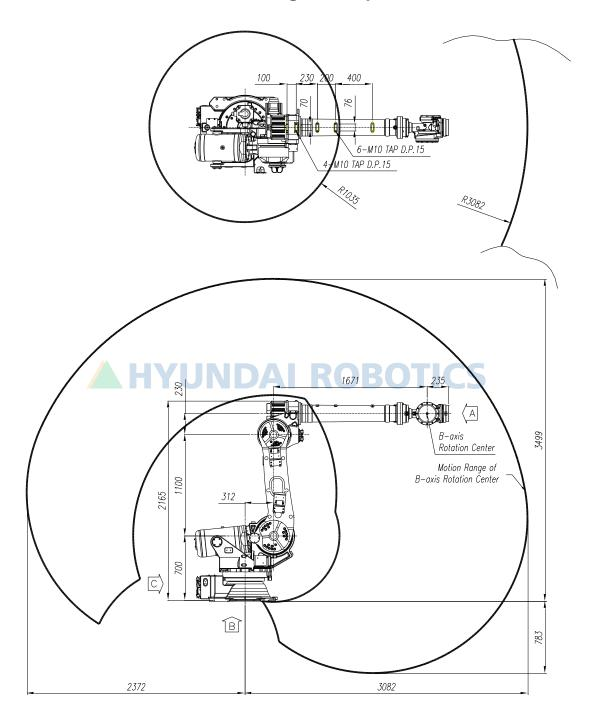
Figure 2.3 Robot Dimension and Working Envelope: [HH130L]
