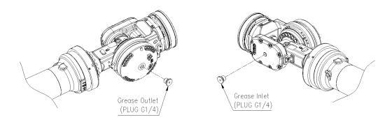
Figure 5.5 B-Axis Reducer Grease Inlet/Outlet
