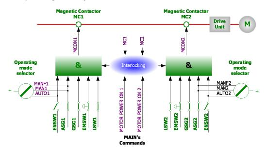
Figure 1.5 Configuration for safety chain
