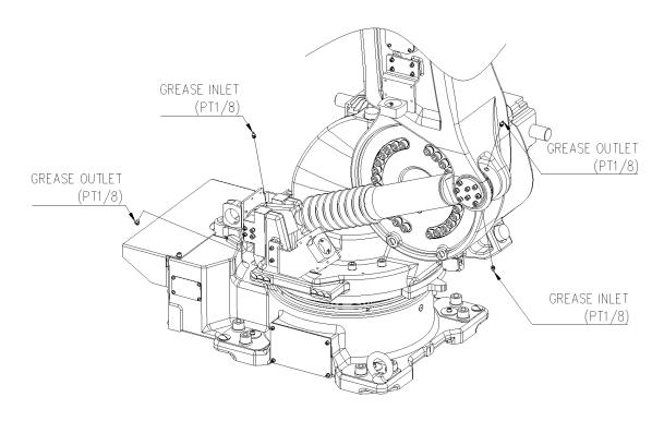
Figure 5.8 Gas Spring Grease Inlet/Outlet (Opening of cover)
