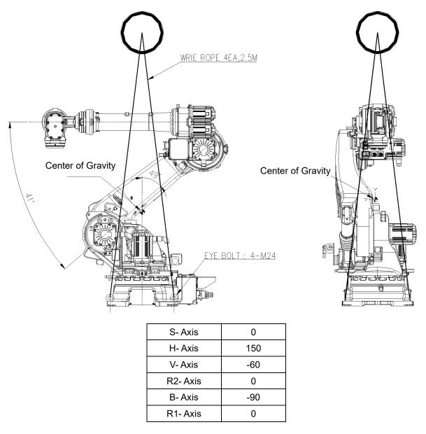
Figure 3.3 How to Transport: Using crane
