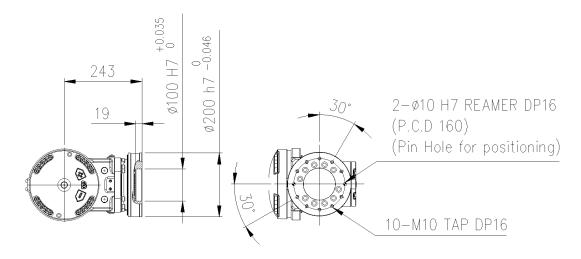
Figure 2.6 Details of Wrist Axis Attachment Surface
