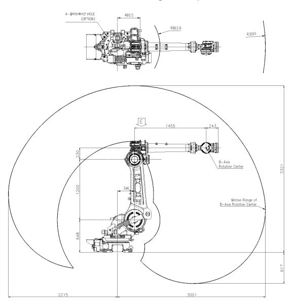
Figure 2.3 Robot Dimension and Working Envelope (HC165L)
