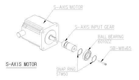
Figure 6.3 Axis S motor assembly
