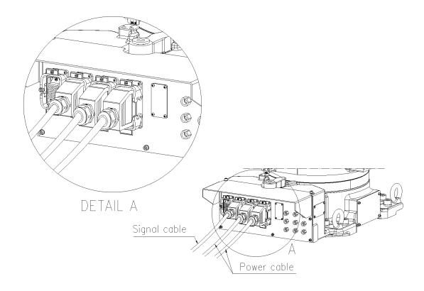
Figure 3.7 Robot Cable Connection
