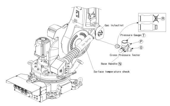
Figure 9.1 Check the Pressure of the Gas Spring
