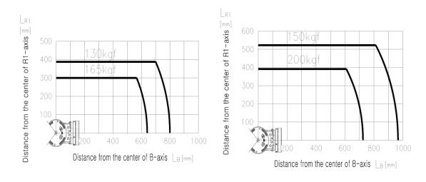
Figure 3.8 Wrist Axis Torque Mapping (Left: HC165L, Right: HC200)
