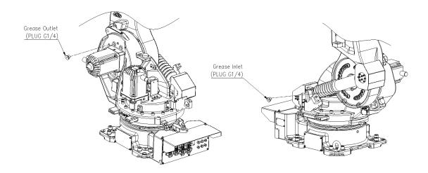
Figure 5.2 H-Axis Reducer Grease Inlet/Outlet
