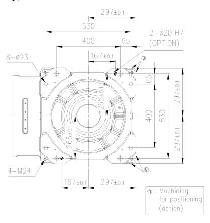
Figure 3.6 Dimension of Robot Installation
