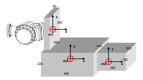
Figure 3.11 3-D load model 3-D shape
