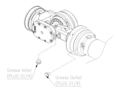
Figure 5.4 R2-Axis Reducer Grease Inlet/Outlet
