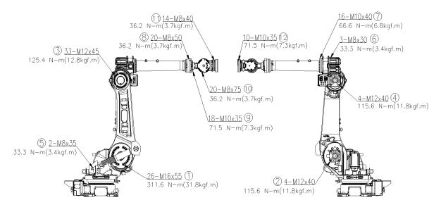
Figure 4.1 Inspection Part for Main Bolts
