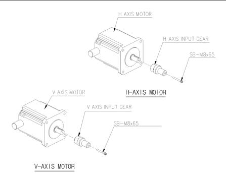
Figure 6.4 Axis H&V Motor Assembly
