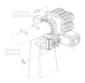
Figure 5.7 Arm Frame Grease Inlet/Outlet
