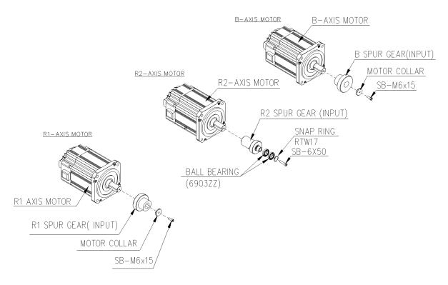
Figure 6.5 Wrist Axis Motor Assembly
