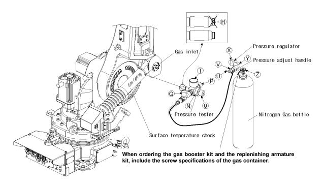
Figure 9.2 Charge Gas into the Gas Spring
