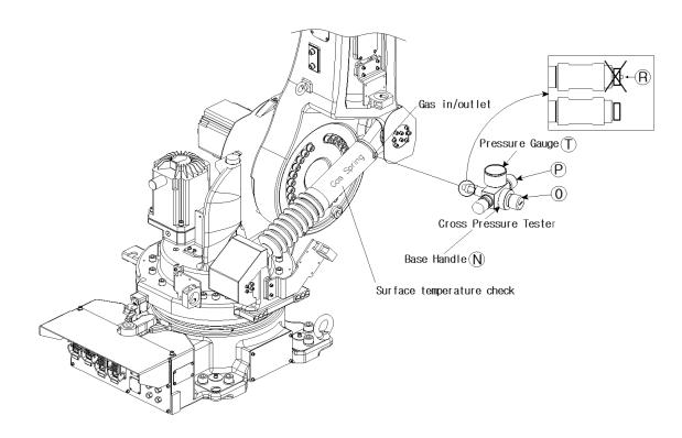
Figure 9.4 Release Gas from the Gas Spring
