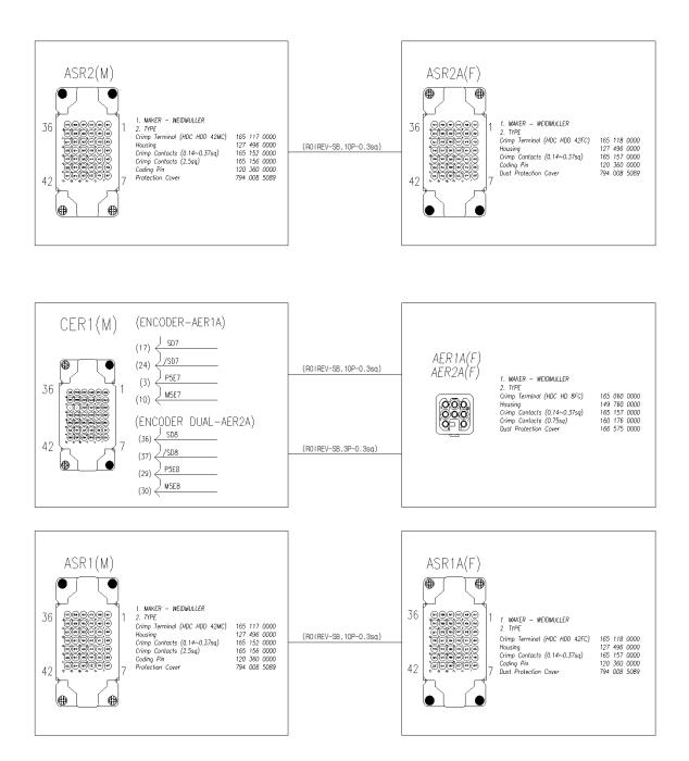
Figure 2.11 Details of Application Connector
