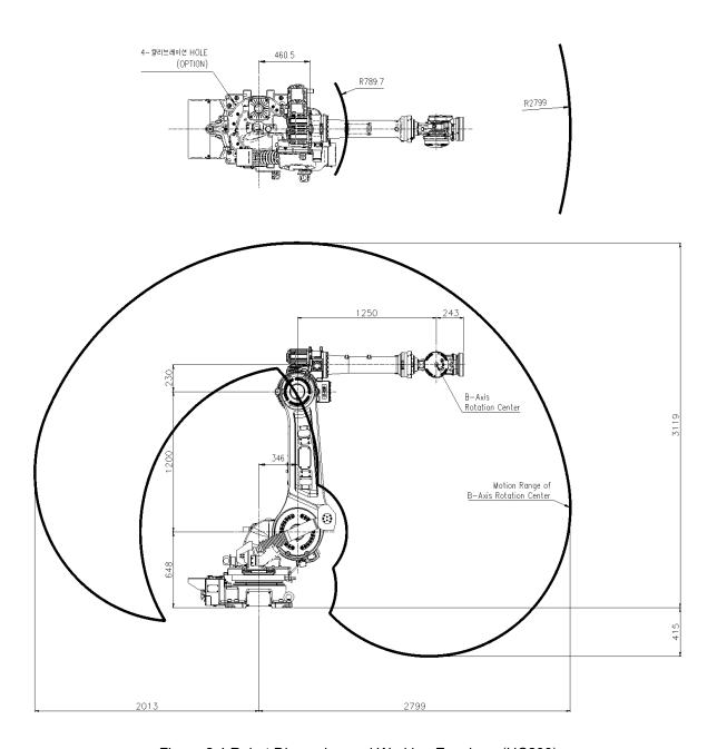
Figure 2.4 Robot Dimension and Working Envelope (HC200)
