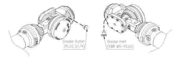
Figure 5.6 R1-Axis Reducer Grease Inlet/Outlet
