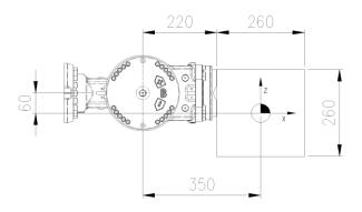
Figure 3.9 2-D load model
