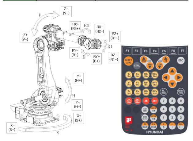
Figure 2.5 Robot Dimension and Axis
