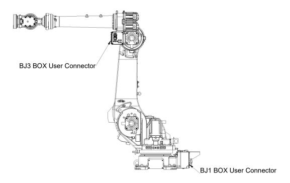
Figure 10.1 Manipulator Configuration
