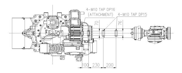
Figure 2.8 Details of Upper ARM FRAME Attachment Surface (HC200)
