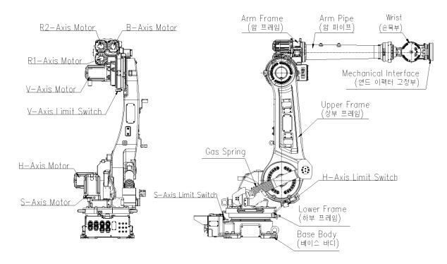
Figure 3.1 Name of Robot Components
