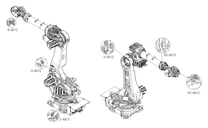
Figure 6.6 Method of Zero Setting
