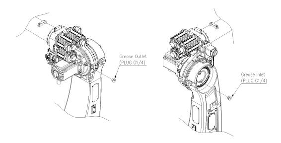
Figure 5.3 V-Axis Reducer Grease Inlet/Outlet
