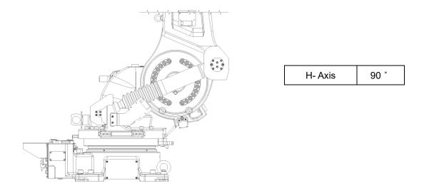
Figure 9.5 Gas spring disassembling posture
