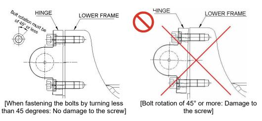
Figure 9.7 Cautions on Fastening and Loosening the Gas Spring Hinge
