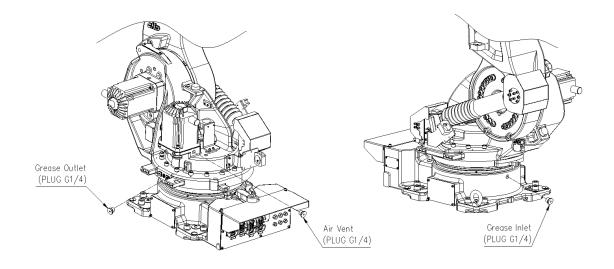
Figure 5.1 S-Axis Reducer Grease Inlet/Outlet
