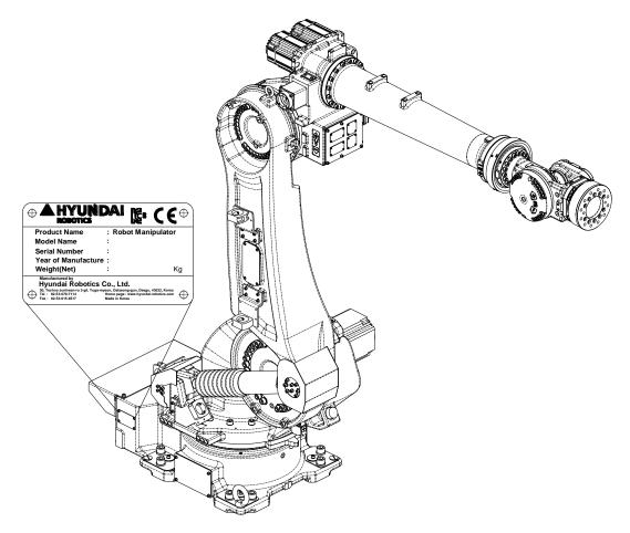
Figure 2.2 The location of identification plate
