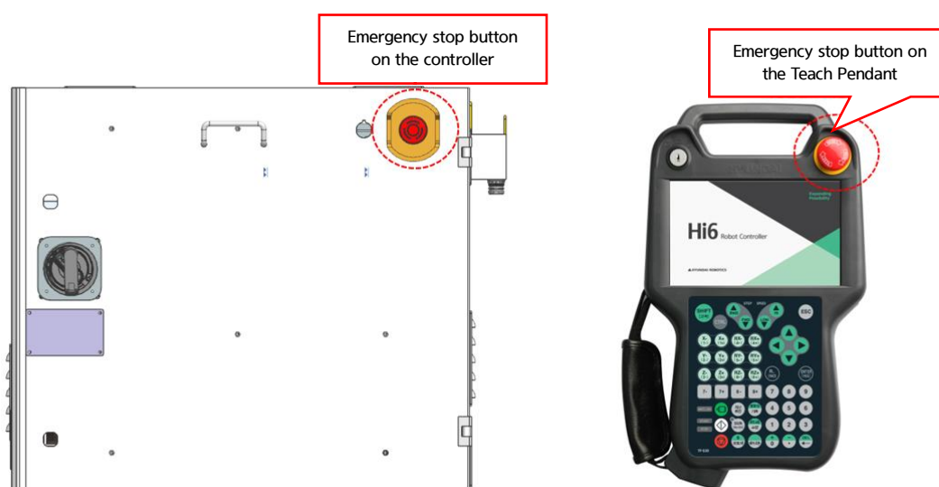
Figure 1.2 Emergency Stop Buttons on the Controller and Teach Pendant
