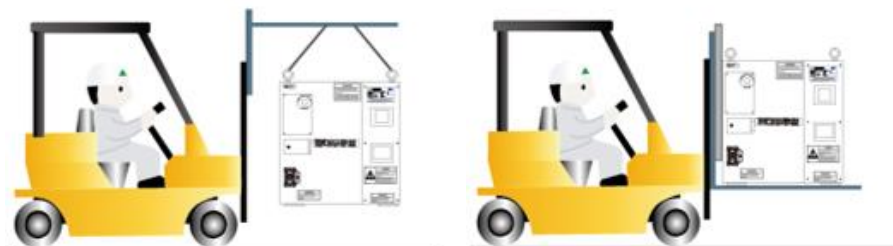
Figure 3.4 Transport of the Controller by Using a Forklift
