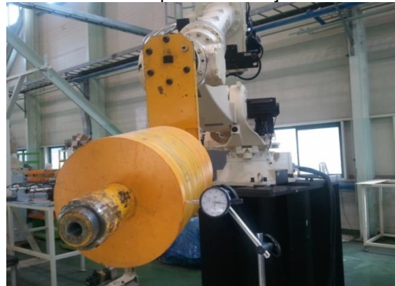
S2 [Origin checkpoint. Only S axis rotates compared with S1]
