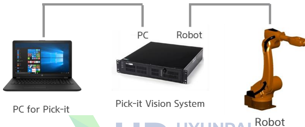
Figure 2-4 Ethernet connection to the Pick-it equipment through TCP
