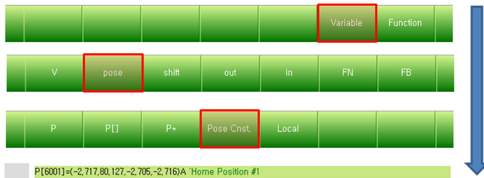
Figure 5.18 Position recording by using pose constant
