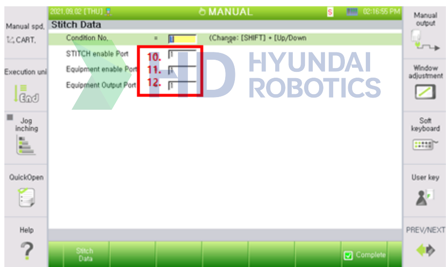
Figure 8.28 Stitch welding parameter setting no. 2
