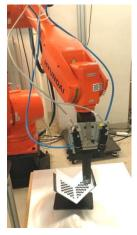
Input the teaching points in the space on the right side in the order of X, Y, and Z, and then press the "Calibration" button to display the transformation matrix and the transformation error. If the error is above 1 mm, then the calibration is incorrect. Camera calibration needs to be performed again. If the error is below 1 mm, click the "Save" button to store the transformation matrix.
