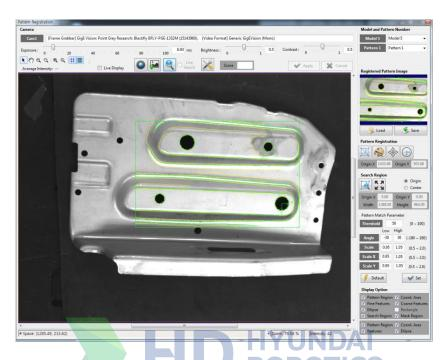
For locating the center of the hole, press the "Find Hole Center" button.
