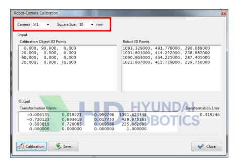
Clicking the "Save" button will store the transformation matrix information into the "C:\text{\psi}HRVision 3D-Stereo\text{\psi}Data\text{\psi}RobCalTransform" folder.
