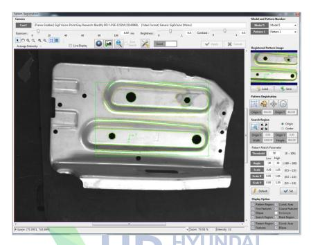
Press the "Apply" button to extract the pattern inside the rectangle.
