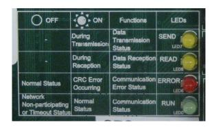
Figure 5.24 LED and Detail of Communication Status Indication of CC-LINK Board (BD570)
