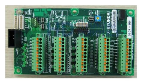
Figure 5.56 Analog/Arc IF Board (BD584)
