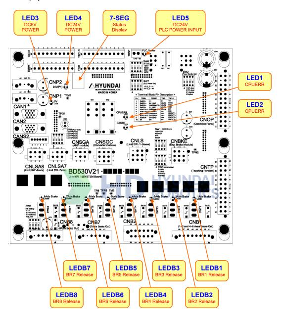
Figure 4.25 The Display Unit of the System Board (BD530)
