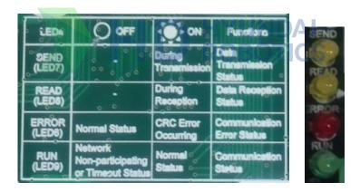
Figure 5. 25 Led For Displaying the Communication Conditions of the CC-link Board (Bd570v20) and the Information
