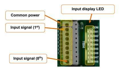
Figure 5.49 Pin Configuration of Digital Input Terminal Block on Expansion Public IO Board (BD583)
