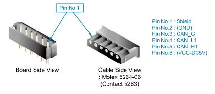
Figure 5.18 Method for Connection of the CAN Connector of the Public IO Board (BD582)
