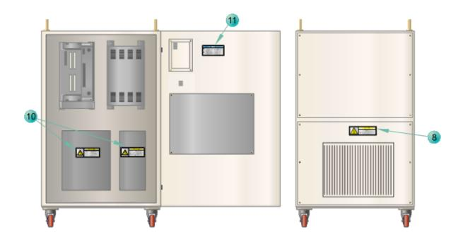
Figure 3.5 Hi5a-C10 Location of Controller Nameplate 2
