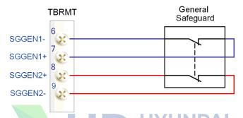
Figure 4.34 Method for connecting a typical safety guard to terminal block TBPLC
