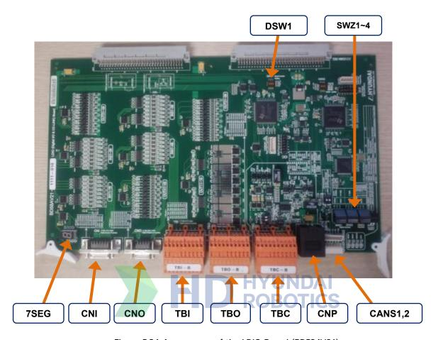
Figure 5.34 Appearance of the LDIO Board (BD58AV21)
