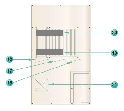
Figure 4.7 Part arrangement in the interior of the rear surface of the Hi5a-N00 controller
