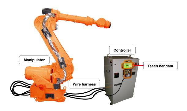
Figure 3.2 Basic Components of Manipulator and Controller (Vertical Articulated Robot)
