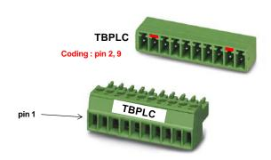
Figure 4.23 System board (BD530) terminal block TBPLC
