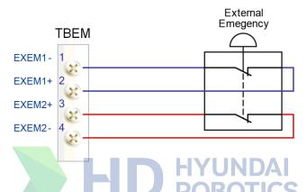
Figure 4.29 Method for connecting the external emergency stop switch to terminal block TBEM
