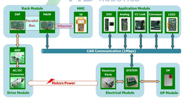
Figure 4.4 Internal Composition of Hi5a Controller
