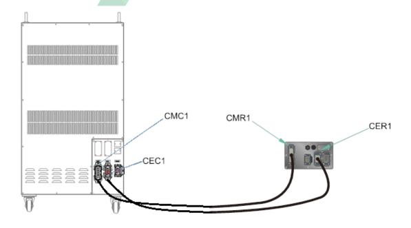
Figure 3.26 Connection of Robot Manipulator and Controller (Hi5a-N30/N50)
