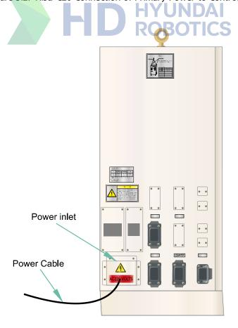
Figure 3.28 Hi5a-C10 Connection of Primary Power to Controller
