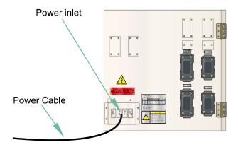
Figure 3.27 Hi5a-C20 Connection of Primary Power to Controller
