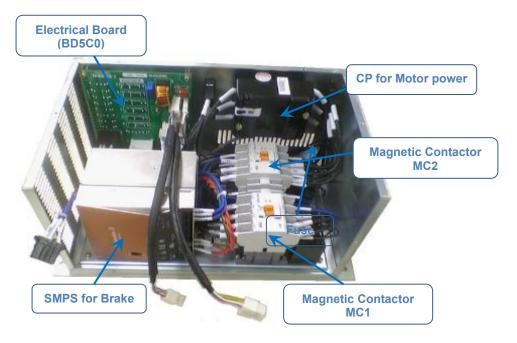
Figure 4.58 The Interior of Electrical Module
