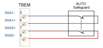
Figure 4.36 Method for connecting the contact point input automatic safety guard to terminal block TBEM
