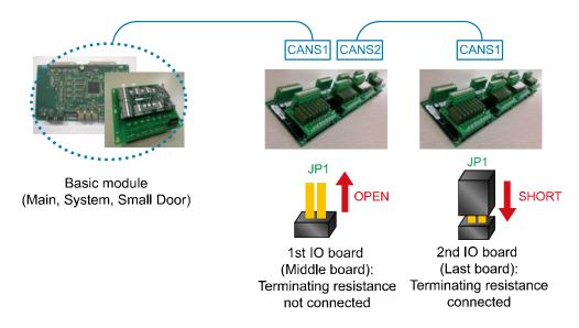
Figure 5.55 Method for Connecting Terminating Resistance
