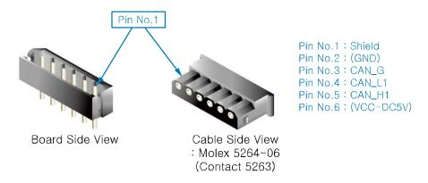
Figure 4.24 Pin arrangement in system CAN connector
