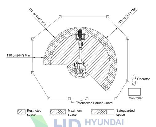
Figure 1.4 Arrangement of general robot peripheral devices and workers
