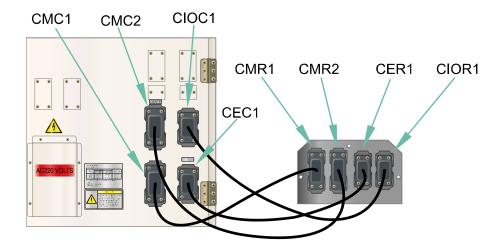
Figure 3.23 Connection of Robot Manipulator and Controller (Hi5a-C20)
