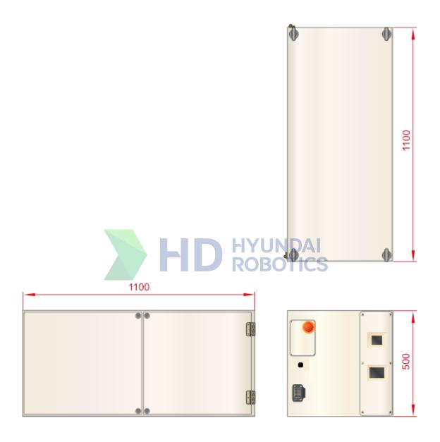
Figure 3.16 Dimension of Hi5a-C20 (Unit: mm)
