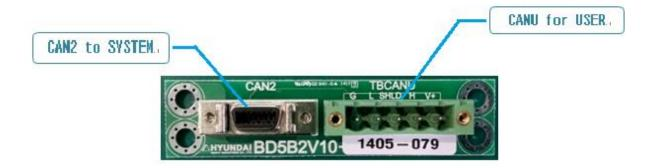
Figure 5. 71 Terminal Board (BD5B2) Configuration
