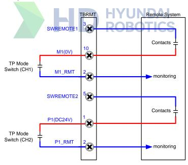
Figure 4.41 for inputting the remote switch signal into terminal block TBRMT
