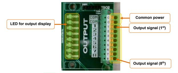
Figure 5.4 Pin Configuration of Digital Input/Output Terminal Block of the Public IO Board(BD580)
