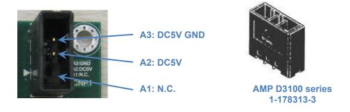
Figure 5.30 Power Connector CNP1 of Conveyor I/F Board (BD585)
