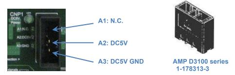
Figure 5.17 Power Connector CNP1 of the Public IO Board (BD582)
