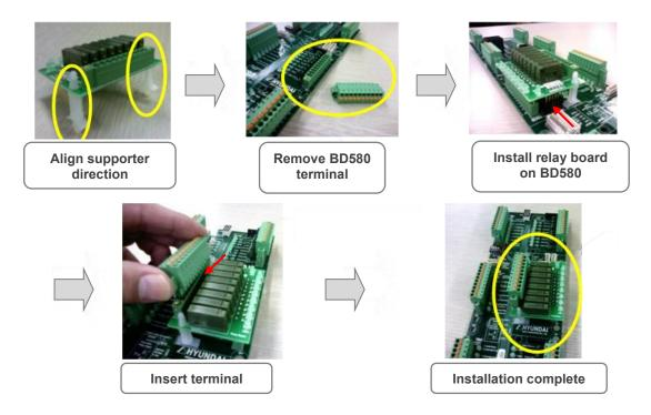
Figure 5.9 Method for the Installation of Relay Board
