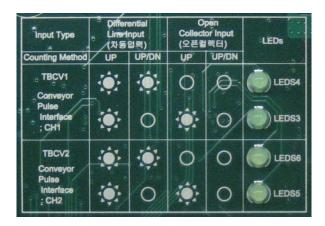
Figure 5.32 LED and Detail for Conveyor I/F Board (BD585) Status Indication
