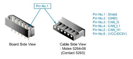
Figure 5.45 Method for Connecting the CAN Connector of LDIO Board (BD58A)
