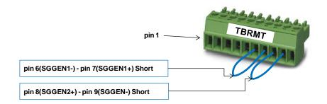
Figure 4.35 Management method in cases where a typical safety guard is not used
