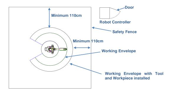
Figure 3.14 Install space for general type robot
