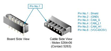
Figure 5.23 Method for the Connection of the CAN Connector of the CC-LINK Board (BD570)
