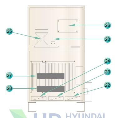
Figure 4.10 Part arrangement in the interior of the rear surface of the Hi5a-C10 controller
