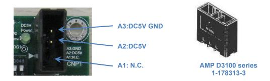
Figure 5.22 Power Connector CNP1 of CC-LINK Board (BD570)
