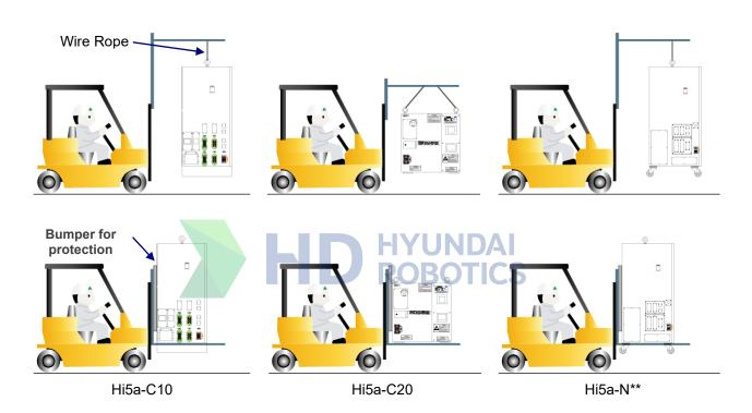
Figure 3.11 Transportation of Controller Using Forklift Truck
