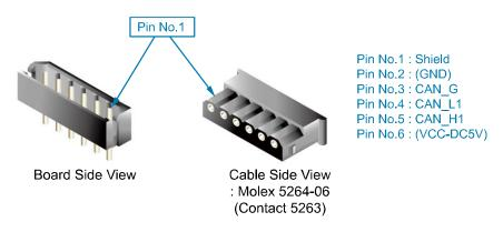
Figure 5.70 Method of Connecting CAN Connector on Analog Board (BD584)
