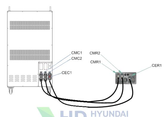
Figure 3.25 Connection of Robot Manipulator and Controller (Hi5a-N00)
