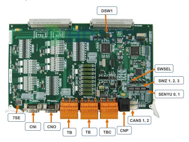
Figure 5.33 Appearance of the LDIO Board (BD58A)
