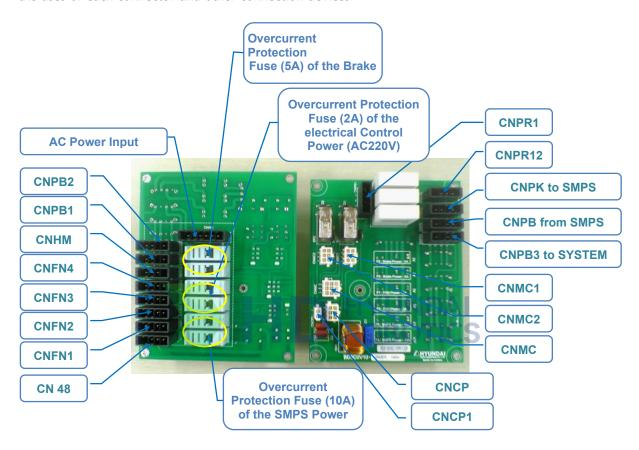
Figure 4.60 Connectors of the Electrical Board (BD5C0)
