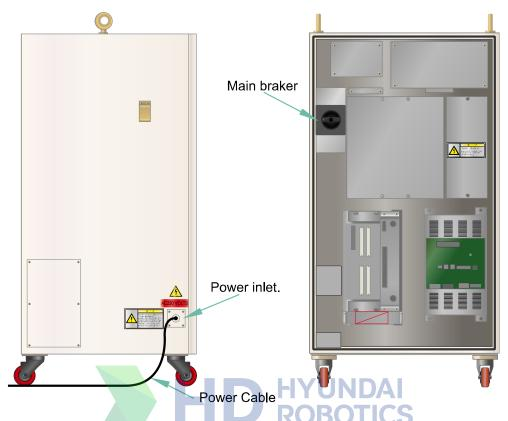
Figure 3.29 Hi5a-N\*\* Connection of Primary Power to Controller
