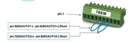
Figure 4.37 Management method in cases where a contact point input automatic safety guard is not used
