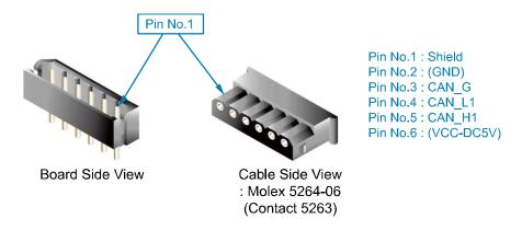
Figure 5.31 Method for the Connection of CAN Connector of the Conveyor I/F Board (BD585)
