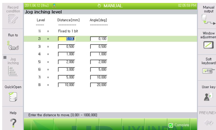
Figure 7.74 Jog inching level setting screen
