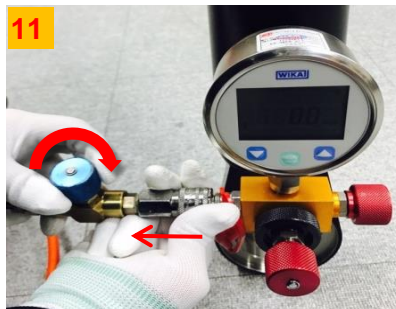
Close the handle of the hose connected to the S86JN (clockwise) and pull out the coupling to disconnect it from the charging plug of the PT118.
