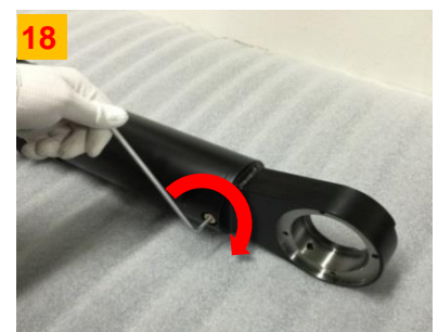
Turn the plug of gas inlet/outlet spring clockwise to tighten it. Make sure to remove any foreign matter on the plug before connecting it.
