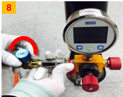
Open the handle of the hose connected to the S86JN (counterclockwise).
