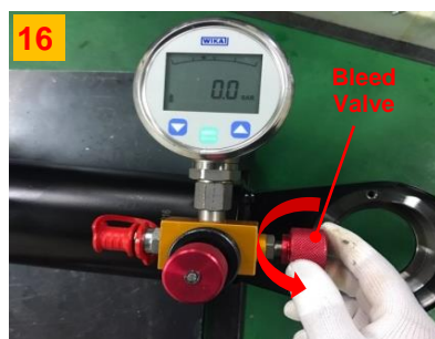
Turn the bleed valve (counterclockwise) to remove residual gas in the PT118.
