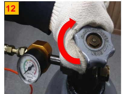
Close the handle of the N2 gas bombe (counterclockwise).
