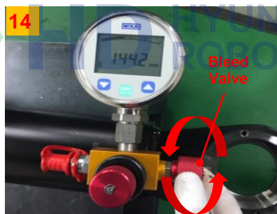
Open and close the bleed valve repeatedly and slowly to set to your desired pressure.
