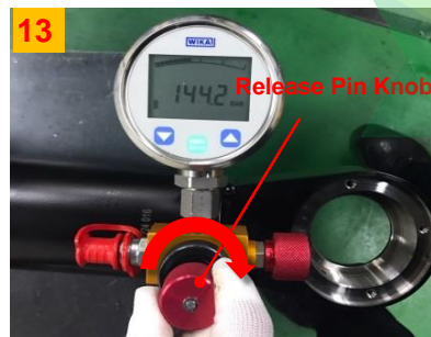
Turn the release pin knob of the PT118 clockwise slowly to check the pressure. (Do not turn the release pin excessively because it will insert the release pin too far and cause damage to the check valve inside the spring.)
