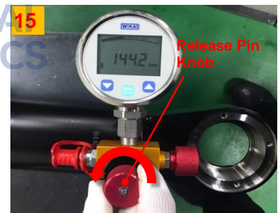
Turn the release pin knob counterclockwise to retract the release pin from the check valve.
