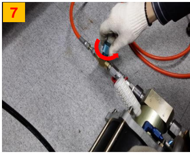
Open the handle of the GCH10 (counterclockwise).
