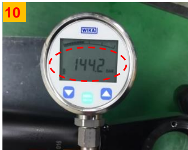
When the defined pressure is reached, close the air valve in step 9 to stop the booster (S86JN).
