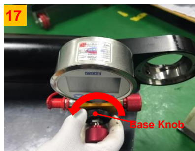
Turn the base knob of the PT118 counterclockwise to separate it from the gas spring.
