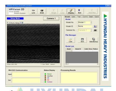
Clicking of the button creates the following "Camera Setup" dialog. Configure "Video Format", "Camera Port", and "Exposure" to fit the installed camera, and click the "Exposure Update" button. The camera 1's port number is 0.
