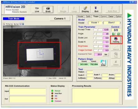
The coordinate axis is arranged at the origin of the pattern, which is set in 4.6.2, and should not be modified by the user using the mouse. In order to modify the coordinate axis position, the 4.6.2 "Pattern Origin" setting process must be conducted.
