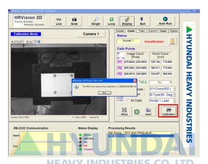
If RMS error is smaller than the "RMS Error Limit" of the "Detail" tab under 3.6.5, the "Setup", the "Input", and the "Calibration" buttons will be activated, and the calibration will be completed. If RMS error is bigger than the "RMS Error Limit" of the "Detail" tab under 3.6.5, a warning dialog will appear and direct the user to perform camera calibration again. Typically, the "RMS Error Limit" is set at 1.
