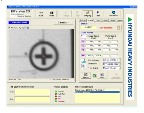
When the search window and coordinate axis are accurately set, click on the "Search" button of the "Calib" tab. The searched results are displayed in the Image window as follows. The "Search" button changes to the "Setup" button. If the search was unsuccessful, re-execute the 4.4.2.4.1 Calibration point detection process
