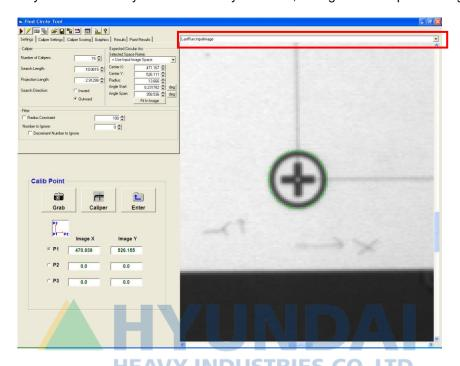
After completing elliptical fitting for the P1 position, perform the same process for P2, and P3.
