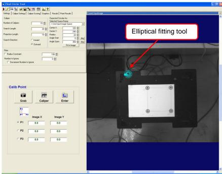
First of all, move the elliptical fitting tool to the P1 position of the image. Right-click on the image to enlarge it. move the correction position
