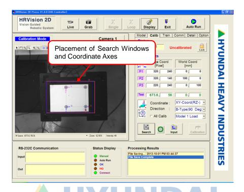
Click on the (Zoom in) of the Image window to expand the calibration board image that has been grabbed.
