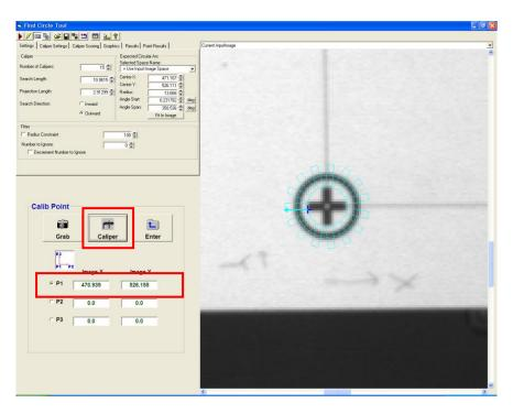
Click the combo box at the upper right part of the "Find Circle Tool" dialog, and select the "LastRun.InputImage". Check whether the outer points of the P1 circle, which are used for elliptical fitting, are correctly detected. If they are not correctly detected, configure the elliptical fitting tool again.
