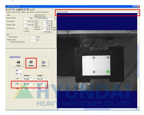
After completing elliptical fitting for the P1 and the P2 positions, perform the same process for P3.
