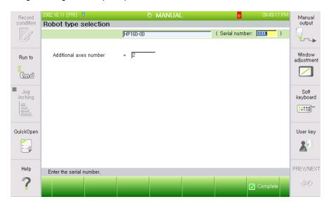
Figure 2.2 Entry of number of additional axes
