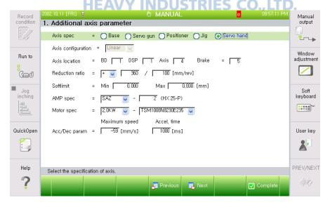
Figure 2.4 Additional Axis Parameter Setting
