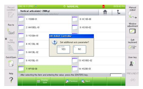
Figure 2.3 Additional Axis Parameter Setting Menu
