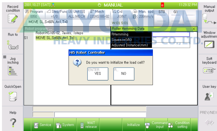
Figure 2.3 Load cell initialization screen
