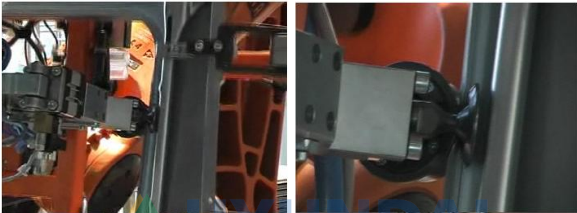
Figure 1.1 Robot roller hemming operation
