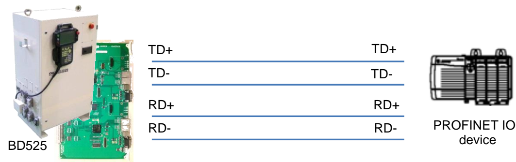
Figure 2.4 Connecting Direct cable
