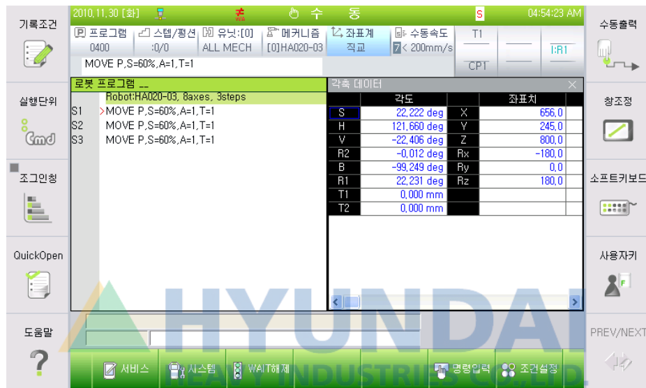
Figure 5.1 Example of the program to set the user coordinate system
