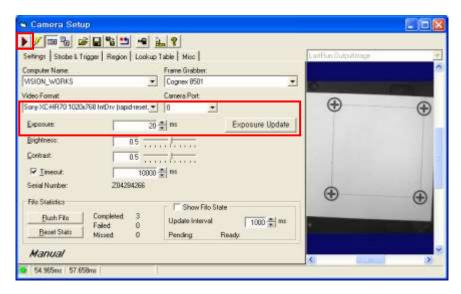
After properly setting the camera, click the button of the "Camera Setup" dialog, and check whether images are normally acquired in the image window placed on the right.
