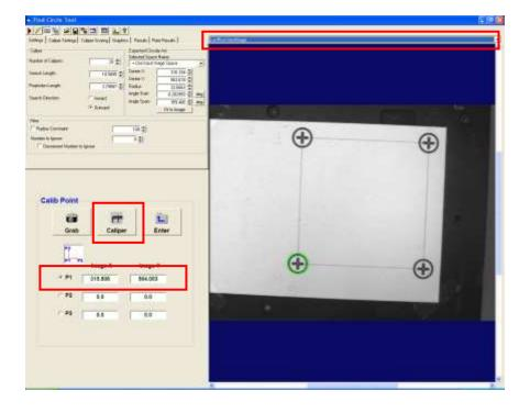
Click the combo box at the upper right part of the "Find Circle Tool" dialog, and select the "LastRun.InputImage". Check whether the outer points of the P1 circle, which are used for elliptical fitting, are correctly detected. If they are not correctly detected, configure the elliptical fitting tool again.
