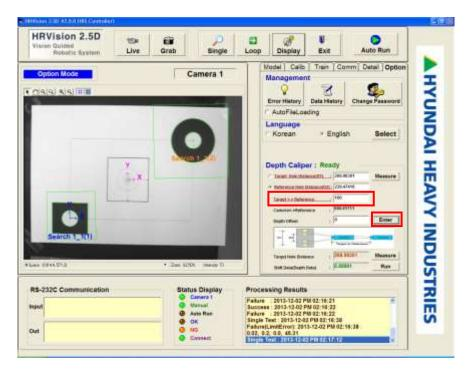
Click the "Run" button, and check whether the "Shift Data (Depth Data)" is measured in the negative sign distance (100mm) in which the robot has been actually shifted.
