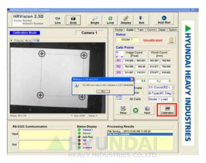
If RMS error is smaller than the "RMS Error Limit" of the "Detail" tab under 3.7.5, the "Setup", the "Input", and the "Calibration" buttons will be activated, and the calibration will be completed. If RMS error is bigger than the "RMS Error Limit" of the "Detail" tab under 3.7.5, a warning dialog will appear and direct the user to perform camera calibration again. Typically, the "RMS Error Limit" is set at 1.
