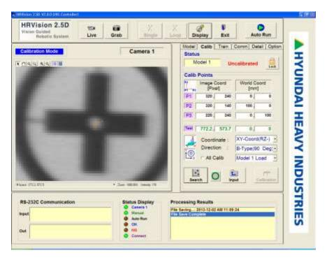
When the search window and coordinate axis are accurately set, click on the "Search" button of the "Calib" tab. The searched results are displayed in the Image window as follows. The "Search" button changes to the "Setup" button. If the search was unsuccessful, re-execute the 4.4.2.4.1 Calibration point detection process
