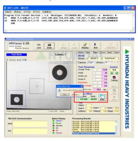
After setup up the pattern setup window and coordinate axis, click on the "Training" button. When the pattern recognition is successful, the following Pattern addition window appears. If there is an error in the pattern recognition, reset the pattern and parameter. Refer to 3.7.3 "Train" tab for parameter setup.
