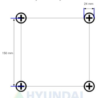
The calibration board is the form of setting the circle with a diameter of 24mm at the corners of a square with a length of 150mm. Refer to the "2D calibration board.dwg" file in the installation CD. Here the 4 circles are called the calibration points, and the calibration work is executed by teaching the central point of this circuit from the image coordinate and the location from the robot coordinate.
