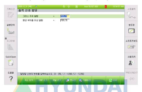
The initial set value is zero (0). It shall be set so that the signal is output outwards. (Note: The allocated signal of grease filling is FB5.DO78)
