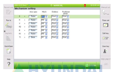
When in manual control mode, the mechanism group of the additional axis should be configured to allocate a jog key according to the mechanism group. Robot axis is locked up as mechanism M0, and additional axis shall be selected by classifying it into mechanisms M1~M7.
