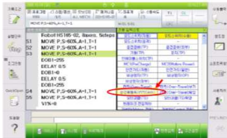
Figure 1.131 Checking the Lift axis belt from Private input signal
