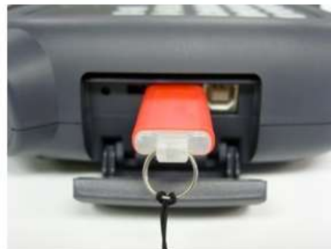
Figure 1.66 Methods for inserting a USB into the teach pendant
