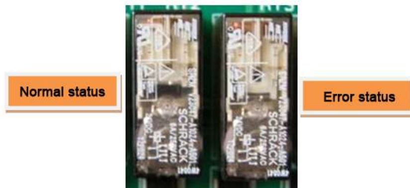
Figure 1.133 Comparing the Normal and Error Status of BD58B Board's Relay
