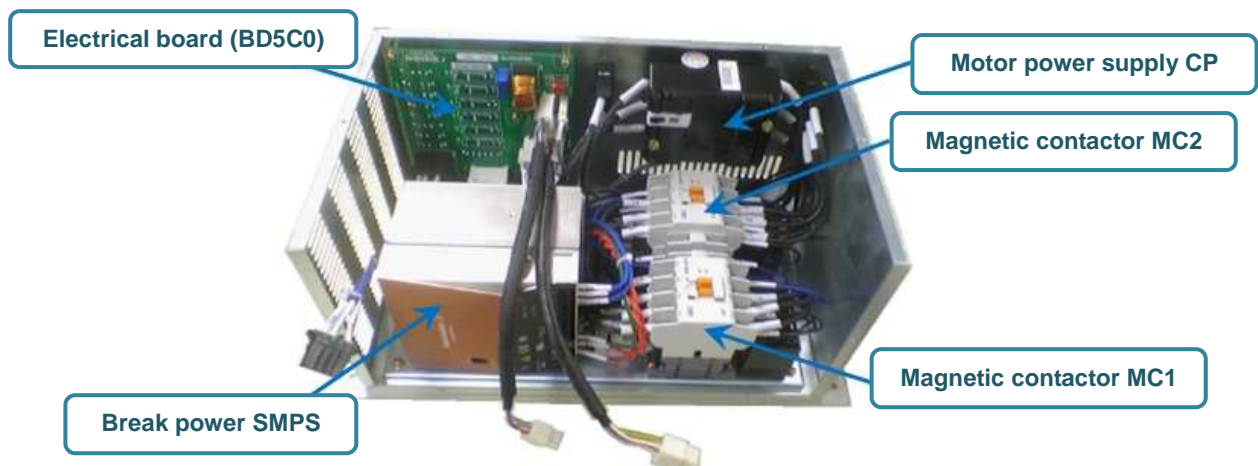
Figure 1.18 Inner Structure of Electrical Module
