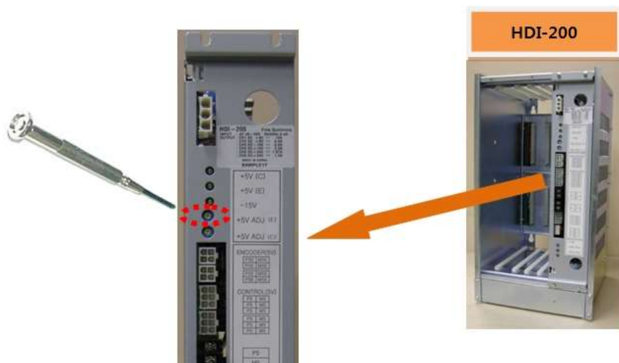
Figure 1.108 Adjusting the encoder voltage
