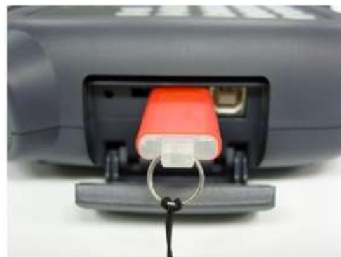
Figure 1.98 Methods for inserting a USB into the teach pendant
