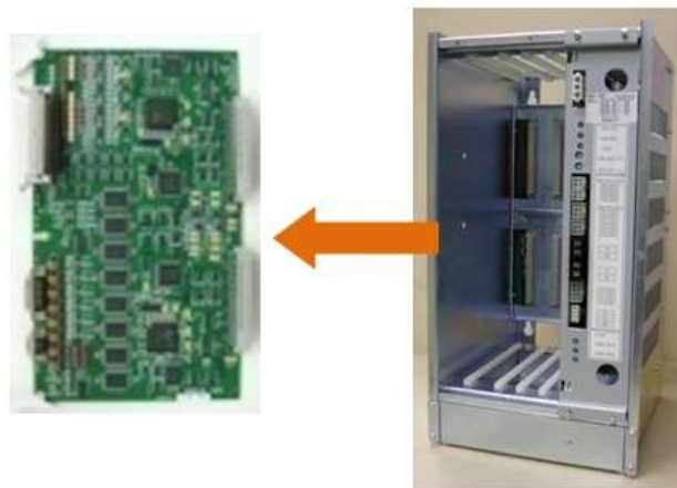
Figure 1.166 Removal of Servo Board from the Rack
