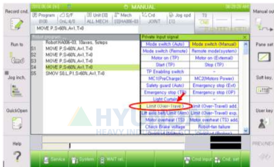
Figure 1.3 Limit (Over-Travel) Monitoring is Displayed from the Private input signal Window
