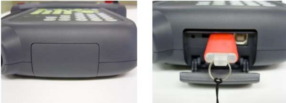
Figure 1.195 Methods for inserting a USB into the teach pendant
