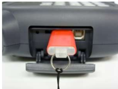
Figure 1.80 Methods for inserting a USB into the teach pendant
