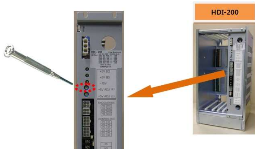
Figure 1.116 Adjusting the encoder voltage
