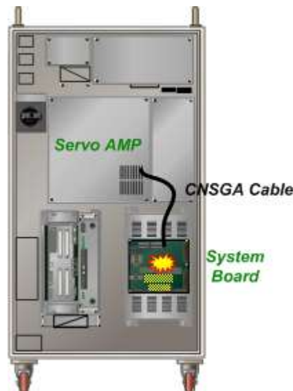
Figure 1.161 Fault with the system board PWMON signal generation circuit
