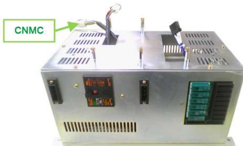
Figure 1.95 CNMC Cable on the Electrical Module
