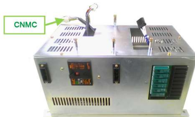
Figure 1.17 CNMC Cable on the Electrical Module
