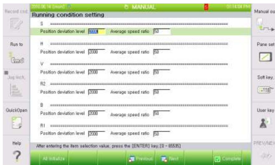
Figure 1.179 Modifying Screen of Position Deviation Value from TP
