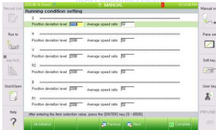
Figure 1.73 Modifying Screen of Position Deviation Value from TP
