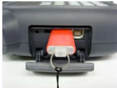
Figure 1.172 Methods for inserting a USB into the teach pendant
