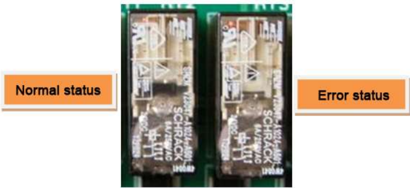
Figure 6.53 Comparing the Normal and Error Status of BD58B Board's Relay
