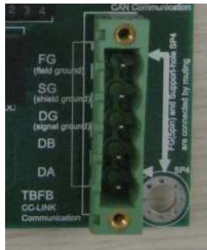
Figure 5.21 CC-LINK Communication Terminal Block of CC-LINK Board (BD570)
