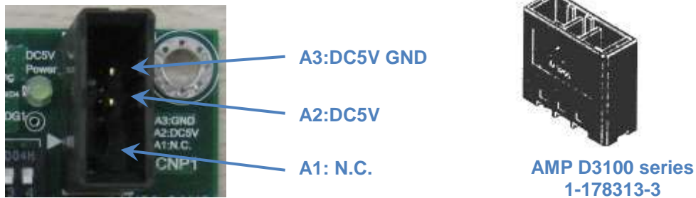
Figure 5.22 Power Connector CNP1 of CC-LINK Board (BD570)
