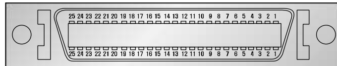
Figure 5.14 CNOOUT Connector (3M MDR 10250-52A2JL) of the Public IO Board (BD582)
