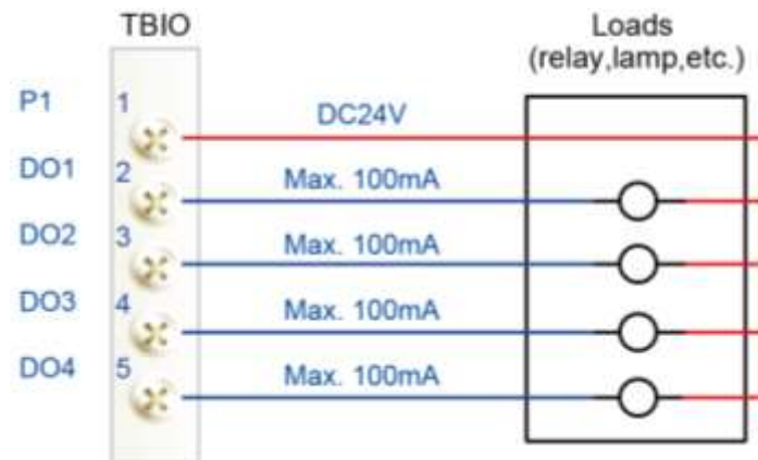
Figure 4.44 Method for connecting digital output for a system to terminal block TBIO
