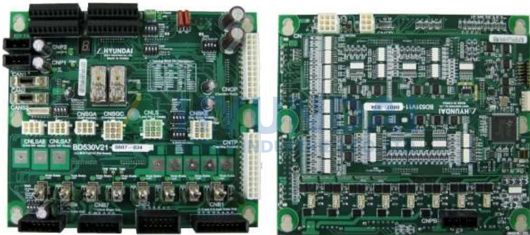
(a) Front: BD530 Board (In charge of sequence) (b) Back: BD531 Board (In charge of system IO)
