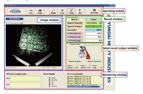
The following picture shows the screen configuration of HRVision (2D) changed to setup mode by clicking on the Tools (Setup) button. With the setup mode, you can setup the vision and manage files. Access is only possible after logging in. The setup window password is notified to the user at the time of purchase for the license of HRVision (2D). The user logs in and changes the password in the option (Option) tab of setup window. Refer to [3.7.5. Option (Option)] tab.
