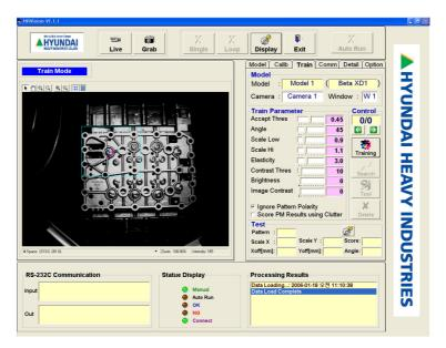
After setup up the pattern setup window and coordinate axis, click on the Train button. When the pattern recognition is successful, the following Pattern addition window appears. If there is an error in the pattern recognition, reset the pattern and parameter. Refer to 3.7.3 Train tab for parameter setup.
