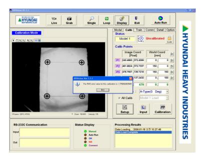
If the RMS error is lower than the RMS Error Limit of 3.7.5. Detail tab, is displays the coordinate axis set to green. If the RMS error is higher than the RMS Error Limit, you will see a warning window to guide you to re-execute the camera calibration. Generally the RMS Error Limit (Permitted RMS error value) is set to standard of 1.
