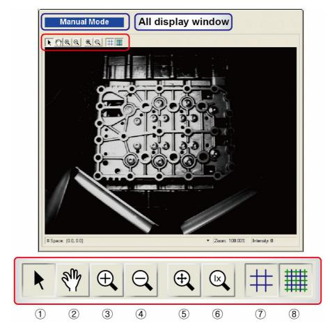
Within the image window, there is the mode display window that shows you all the currently executed modes, and the operating tool mode that will help you efficiently view the grabbed image. HRVision (2D) has largely 3 modes, the manual mode, the run mode and the setup mode, and the setup mode has 6 modes, model setup, calibration, train, communication setup, DIO and option.
