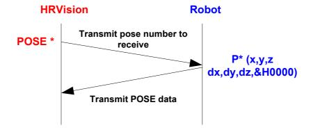
The following code is a robot work code to transmit the POSE data of the robot automatically in connection with HRVision (2D). The user generates the new robot work program and insert the following code as is. To receive the POSE data of the robot automatically, the robot work program must be in operation from the robot controller.
