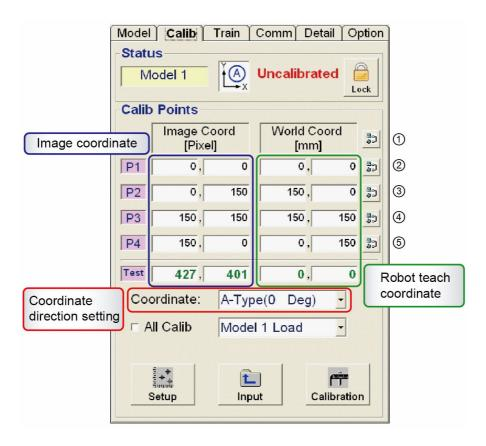
The detail description of Calib tab is as follows.
