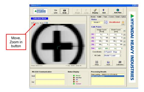
When the search window and coordinate axis are accurately set, click on the Search button of the Calib tab. The searched results are displayed in the Image window as follows. The Search button changes to the Setup button. If the search was unsuccessful, re-execute the 4.5.2.4. Calibration point detection process.
