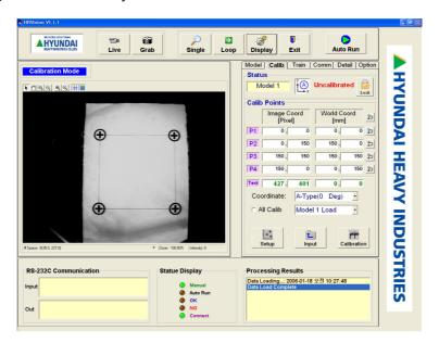
Enter the camera direction for the robot coordinate. Refer to 3.7.2 Calib for details.
