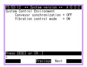
See chapter 4 about On/Off function of vibration controller when On/Off of vibration controller needs to change according to the vibration and the trajectory feature of robot as the teaching about robot operation is completed.
