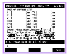
(2)  $\llbracket [PF2]$ : System $\rrbracket \to \llbracket 1$ : User parameter $\rrbracket \to \llbracket 2$ : Pose REC type = <Base, Robot, Enc,  $\fbox{U}, \fbox{Un} > \rrbracket$
