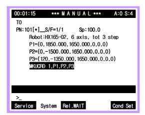
The above instruction is to register the user coordinate using pose variable and the location can be detected by sensor and can register the user coordinate by online.
