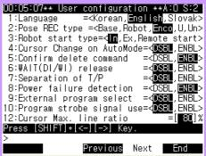
Set up to "U" and "UN" at "2: Pose REC type = <Base,Robot,Enco,U,Un> from above screen.
