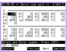
Set each gain of the servo controller. If servo loop gain is changed, this immediately affects the servo controller. Therefore, it is safe to change the gain when motor is off.
