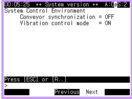
Since the vibration controller controls the robot based on robot dynamics, load data of tool is necessary to improve control performance.
