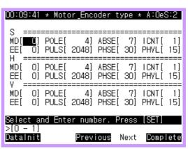
Set parameters according to the type of motor and encoder.
