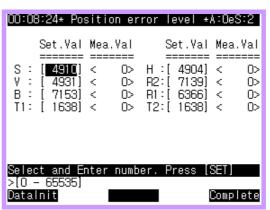
Set a deviation value to detect axis deviation error <code>"E0117 oAx)</code> Too large position drift when unusual moves are found in robot performance.
