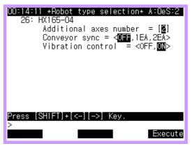
Also, after the initialization is completed, go to  $\lceil [PF1] : Service \rfloor \rightarrow \lceil 7 : System checking \rfloor \rightarrow \lceil 1 : System Version \rfloor \rightarrow \lceil [PF4] : Next \rfloor$  to check vibration controller availability.
