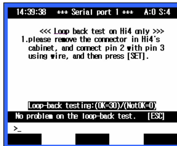
Fig. 4.12 Normal result of RS-232C communication test
