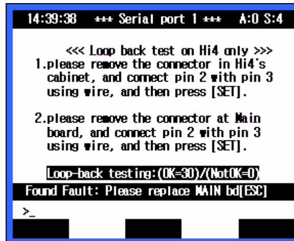
Fig. 4.15 Result when the RS-232C of the main board abnormally functions
