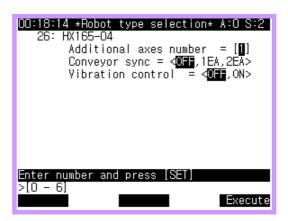
(3) Set servo parameter for gun no.1 (servo gun no.1) through additional axis constant setting.
