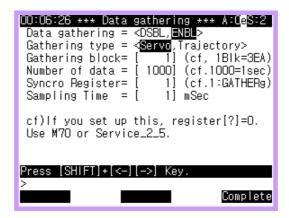
Enter the data as required from the above screen and press  $\lceil [PF5] \rceil$ : Complete  $\lceil key \rceil$  key. It will create a data collection file (ROBOT.GT0). Set it up as explained in the next section and start the arc sensing to collect the data related to arc sensing. Collect data number, from above, is not 1000=1 sec but 1 per 10msec. Therefore it is 1000/(1000/10)=10 sec.
