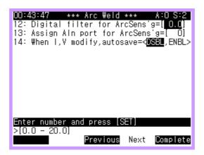
You can set the welding current input port using the menu item 13 from above. If the from the above menu. If "Arc sensing =<Enable>\_ from the arc sending condition to be explained later, is allocated to the value of 0, it will indicate an error saying "E1296 Assign InPORT of weld [A] for TRK.\_ and stop.
