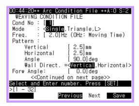
(2) Press <sup>[[PF3]</sup>: Next<sub>]</sub> twice from the above screen to see the following arc sensing condition.
