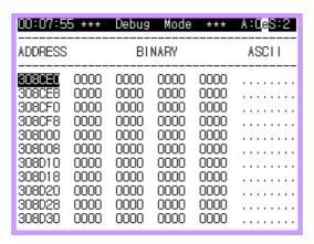
(2) Enter 4080010E (Refer to below A~F input method) and press the [SET] key. You can see the screen change as follows.
