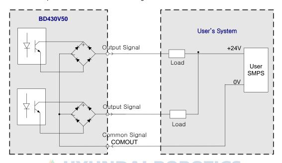
Fig. 4.13 BD430V50 Board Schematic Diagram(NPN voltage output type)
