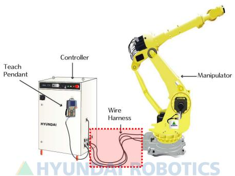
Fig. 5.36 Basic installation diagram between the robot and the controller.
