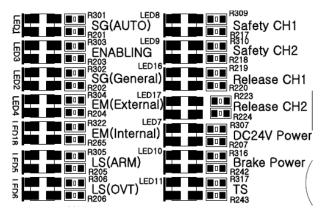
Fig. 4.38 Safety signal LED of sequence board (BD461V50/60)
