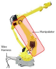
Fig. 5.53 Robot's internal wiring
