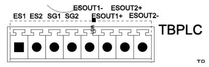
Fig. 4.35 Pin diagram of terminal block TBPLC
