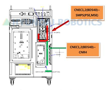
Fig. 5.43 controller's internal encoder wiring
