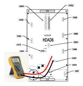
Fig. 5.51 Short-circuit test on the switching device of HDAD6
