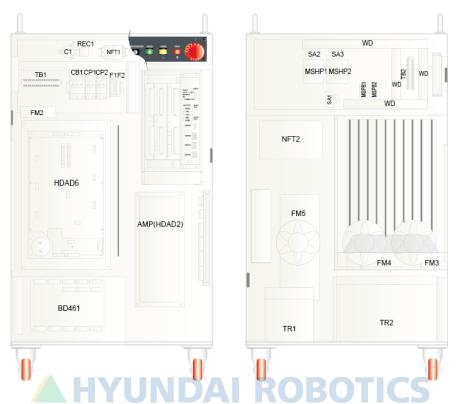
Fig. 4.2 Parts Configuration of Hi4a-0002, Hi4a-0012 Controller
