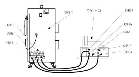
Fig. 5.45 Connection between the robot's main frame and the controller
