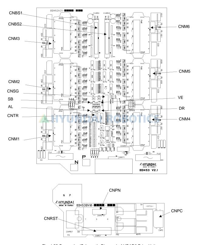
Fig. 4.55 Connection(Schematic Diagram) of HDAD6 Drive Unit
