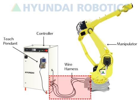
Fig. 5.52 Basic installation diagram between the robot and the controller
