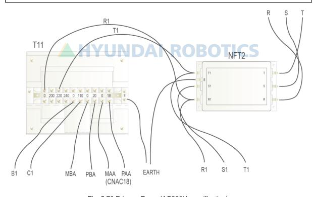
Fig. 5.70 Primary Power(AC220V specification)
