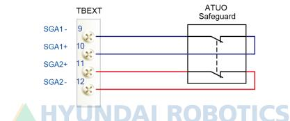
Fig. 4.33 Connection of AUTO safety guard switch of terminal block TBEXT
