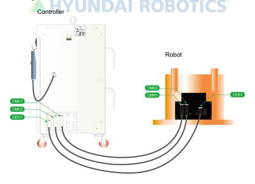
Fig. 3.17 Connection of Robot Manipulator and Controller (Hi4a-0010)
