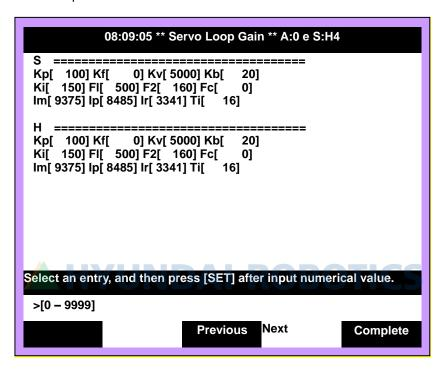
If the vibration occurs at the tip of robot tool, increase F1 and F2 of servo parameters with the same ratio for all axes. For instance, to increase by 20% with F1=500 and F2=160 as above, change them to F1=600 and F2=192 for all axes.
