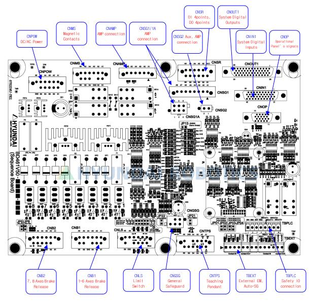
Fig. 4.30 Connector arrangement of sequence board (BD461V50/60)
