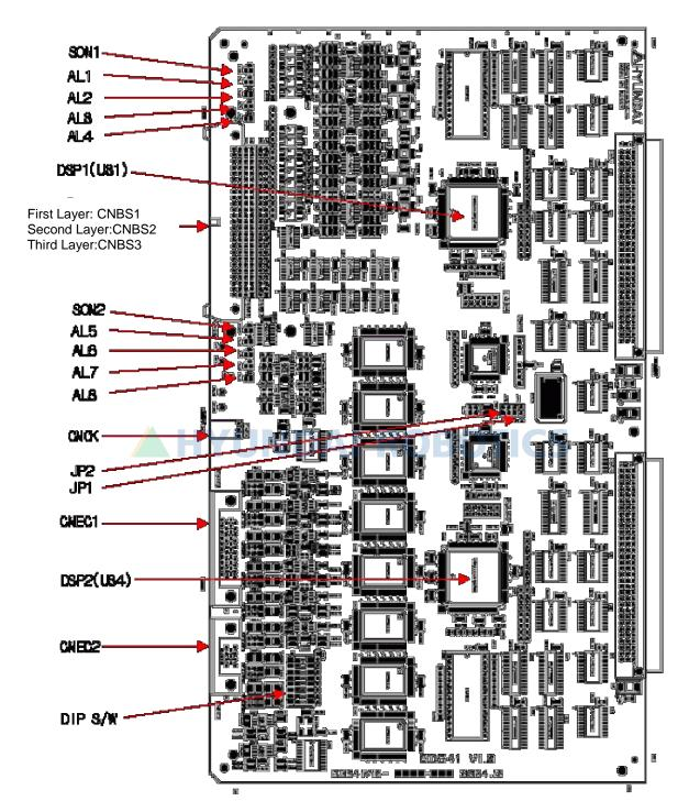
Fig. 4.20 Exterior View of BD541 Board
