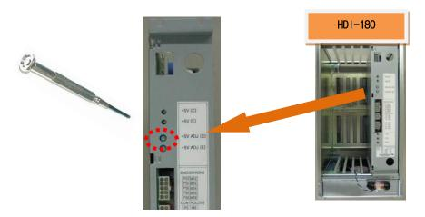
Fig. 5.32 How to adjust the power of the encoder
