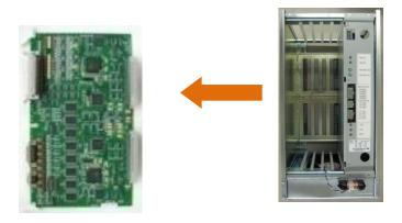
Fig. 5.60 Removal of the Servo board from the rack
