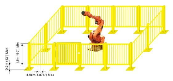
Fig. 1.2 Recommended Size for Fence and Gate Hole (Slot Gate)
