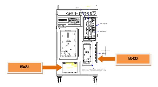
Fig. 5.15 Replacement of the Hi4a-0010/0012 controller's BD461/BD430
