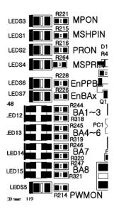
Fig. 4.39 Motor/brake power LED of sequence board (BD461V50/60)
