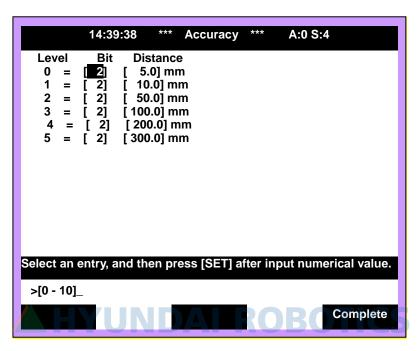
If the accuracy is 0 for the step in which the problem occurred, increase the bit and distance of Level 0 into a level allowed for the operation.
