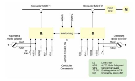
Fig. 5.64 Concept diagram of the safety circuit for the motor's power on/off
