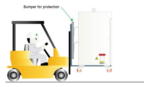
Fig. 3.8 Transportation of Controller Using Forklift Truck
