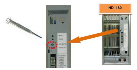
Fig. 5.22 How to adjust the power of the encoder
