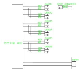
Fig. 5.30 Connector for resetting of the encoder
