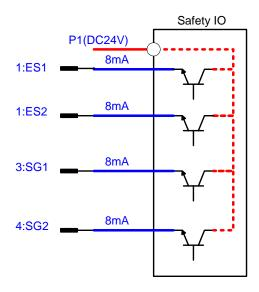
Fig. 4.36 NPN type safety guard connection method and general safety guard connection
