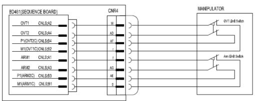
Fig. 5.3 Wirings that are related to a limit switch status input
