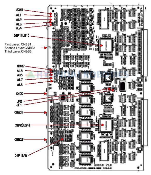
Fig. 4.19 Exterior View of BD540 Board
