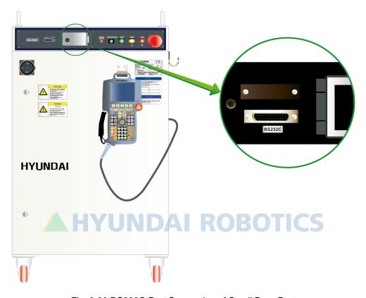
Fig. 3.20 RS232C Port Connection of Small Door Part
