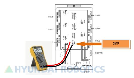
Fig. 5.6 Measuring the resistance value from the Hi4a-0000 controller's CNTR
