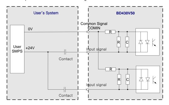
Fig. 4.10 Schematic Diagram(PNP voltage output type)
