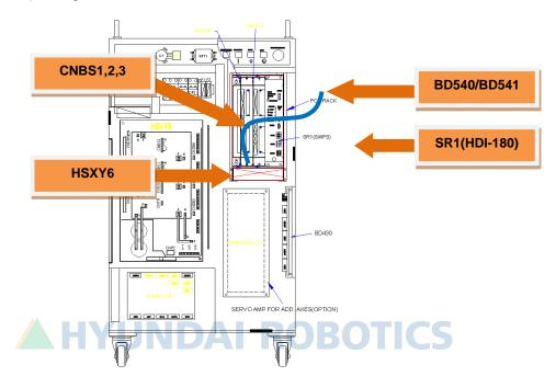
Fig. 5.56 Locations of the components in the Hi4a-0000 controller that are related to the drive unit control voltage reduction
