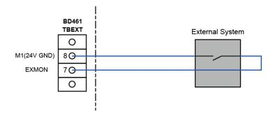
Fig. 4.26 Connection of External Motor ON Input
