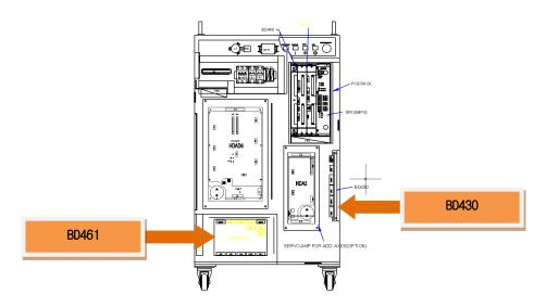
Fig. 5.9 Replacement of the Hi4a-0010/0012 controller's BD461/BD430
