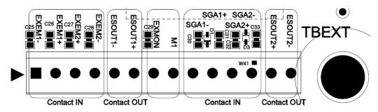
Fig. 4.31 Pin diagram of terminal block TBEXT
