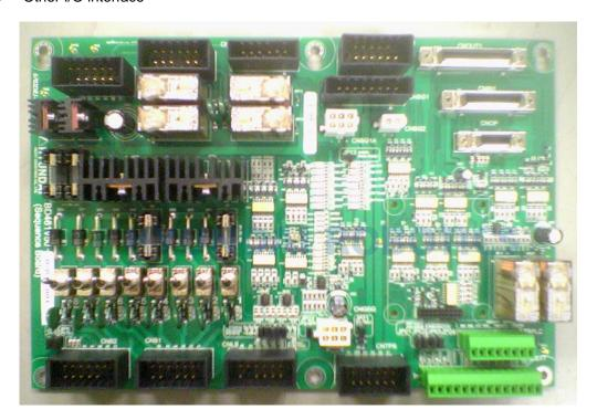
Fig. 4.29 Sequence board (BD461V50) exterior
