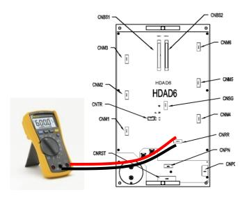
Fig. 5.17 Measuring the resistance value from the Hi4a-0010/0012 controller's CNKPPN
