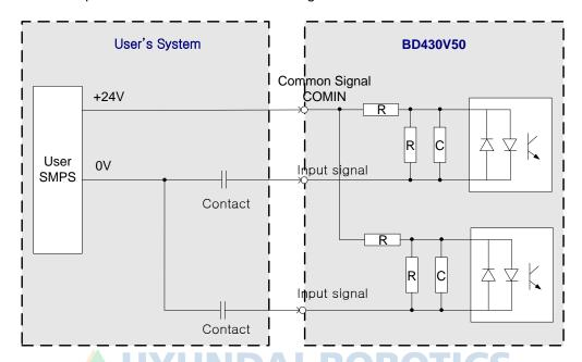
Fig. 4.9 Schematic Diagram(NPN voltage output type)
