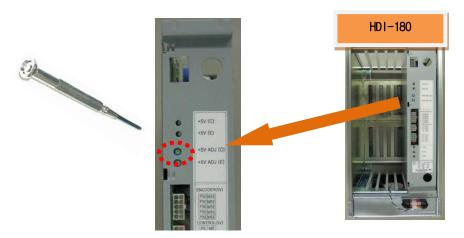
Fig. 5.40 How to adjust the power of the encoder
