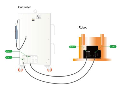
Fig. 3.18 Connection of Robot Manipulator and Controller (Hi4a-0012)
