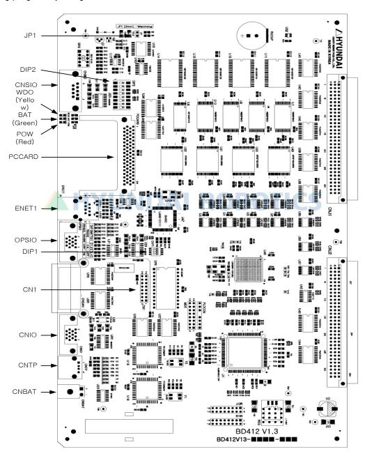
Fig. 4.5 Main Board (BD412) Exterior View
