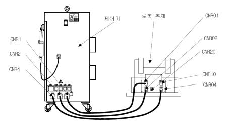
Fig. 5.37 Connection between the robot's main frame and the controller
