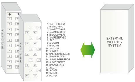
Fig. 4.46 CNWIF connector Specifications
