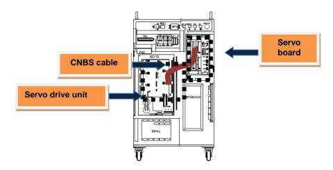
Fig. 5.55 Controller internal side (CNBS cable)
