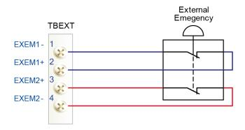
Fig. 4.32 Connection of external emergency stop switch of terminal block TBEXTF
