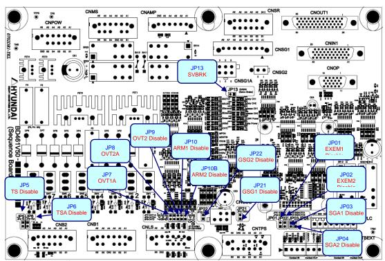
Fig. 4.40 Setup device of sequence board (BD461V50/60)
