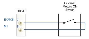
Fig. 4.34 Connection of external motor power ON signal input of terminal block TBEXT
