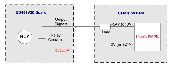
Fig. 4.48 CNWIF Output Signal Connecting Method
