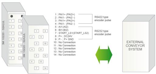
Fig. 4.49 CNCP1, 2 Connector Specifications
