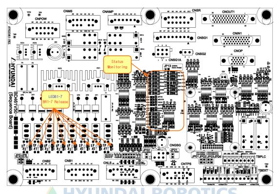
Fig. 4.37 Label device of sequence board (BD461V50/60)
