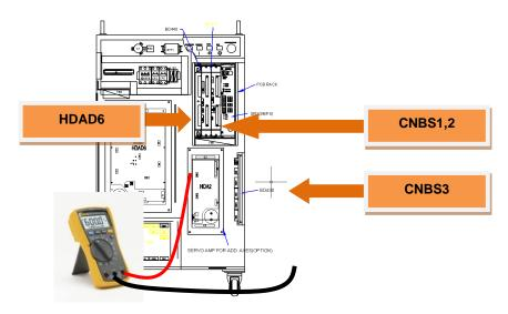
Fig. 5.49 Examining the output cable of the Servo drive unit (Hi4a-0010/0012)
