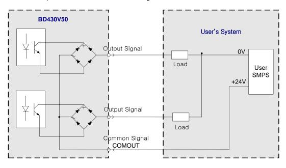
Fig. 4.14 BD430V50 Board Schematic Diagram(PNP voltage output type)
