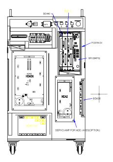
Fig. 5.13 Locations of components in the Hi4a-0010/0012 controller that are related to the overvoltage occurrence error
