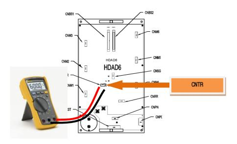
Fig. 5.7 Measuring the resistance value from the Hi4a-0012/0012 controller's CNTR
