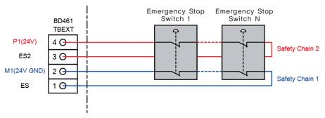
Fig. 4.24 (a) Connection of Emergency Stop Switch in External System
