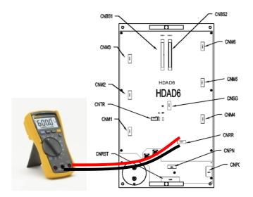
Fig. 5.11 Measuring the resistance value from the Hi4a-0010/0012 controller's CNKPPN
