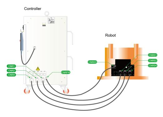
Fig. 3.16 Connection of Robot Manipulator and Controller (Hi4a-0008)
