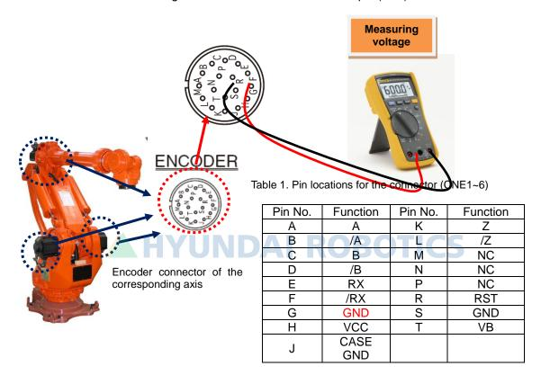
Fig. 5.39 How to measure the input power of the encoder
