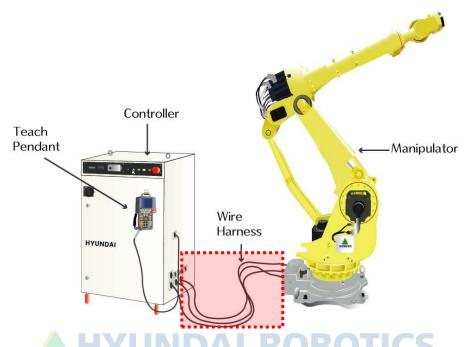
Fig. 5.44 Basic installation diagram between the robot and the controller.
