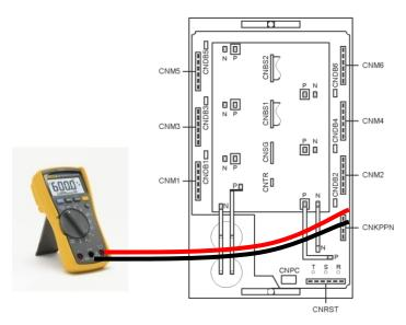
Fig. 5.16 Measuring the resistance value from the Hi4a-0000 controller's CNKPPN
