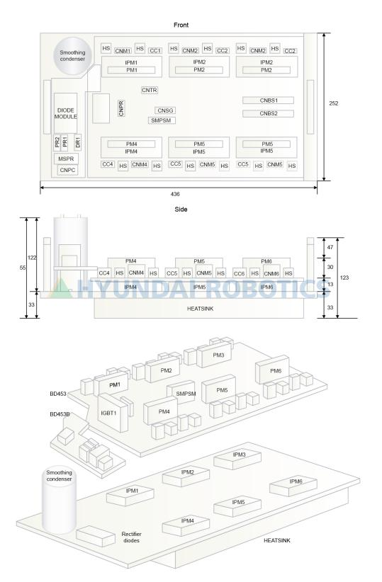
Fig. 4.54 Exterior View of HDAD6 Drive Unit
