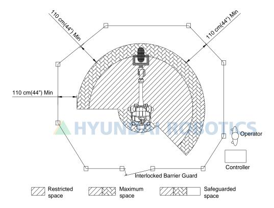
Fig. 1.3 Placement of Peripheral Equipment and Operator
