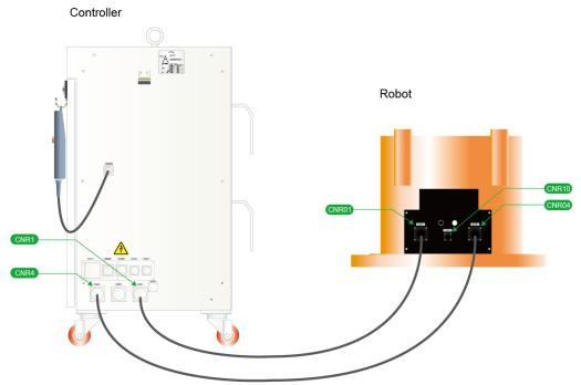
Fig. 3.15 Connection of Robot Manipulator and Controller (Hi4a-0002)
