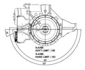
Fig. 5.2 Operation area for the S-axis limit switch
