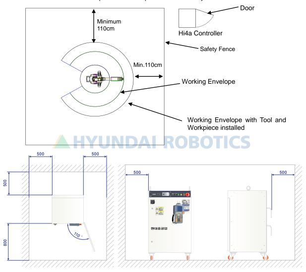
Fig. 1.4 Space for robot installation
