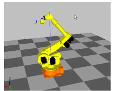
Fig. 5.67 Axis S singular point
