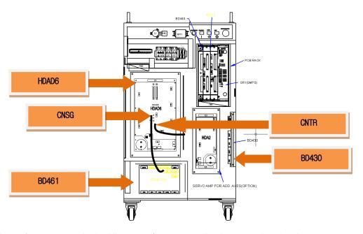
Fig. 5.5 Locations of components in the Hi4a-0010/0012 controller that are related to the recovery resistance overheat error
