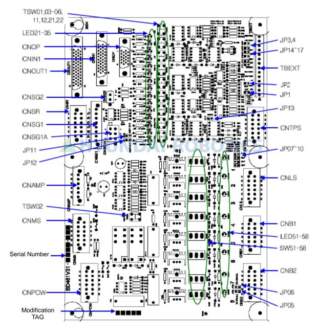
Fig. 4.21 Exterior View of Sequence Board(BD461)
