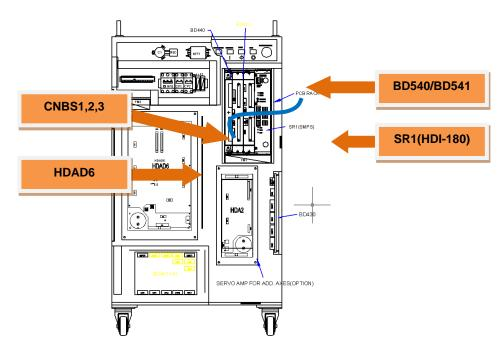
Fig. 5.57 Locations of the components in the Hi4a-0010/0012 controller that are related to the drive unit control voltage reduction
