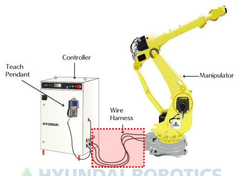
Fig. 5.27 Basic installation diagram between the robot and the controller.
