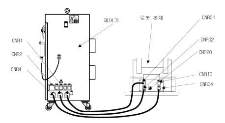
Fig. 5.28 Connection between the robot's main frame and the controller
