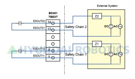
Fig. 4.25 (b) Connection of Emergency Stop Output to External System
