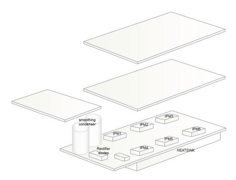
Fig. 4.51 Exterior View of HSXY6 Drive Unit
