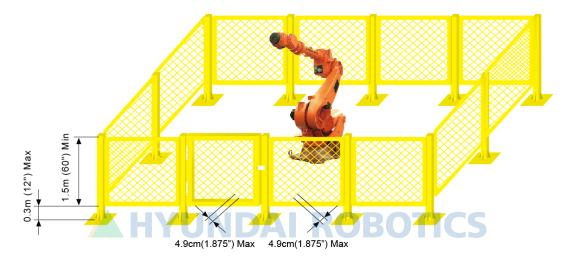
Fig. 1.1 Recommended Size for Fence and Gate Hole (Square Gate)
