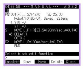
(4) Move the cursor to the line right before the line to copy by using the [Arrow] key. (45 DELAY 1 line)
