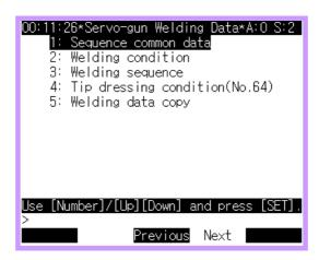
(2) Enter into sub-menu if pressing after pressing the [SET] key aft er moving a reverse bar with the [Direction] key to the item to select, or inputting number of the item to select into the Input frame with the [NUMBER] key.
