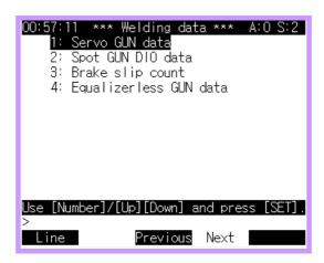
(2) Press the [SET] key after selecting desired item by using with the [Number] key or arrow key.
