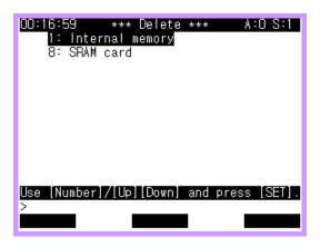
(3) Selection the file to be deleted, and press  $\lceil [PF5] \rceil$ : Execute\_ $\rfloor$ . Refer to the Reference of  $\lceil 4.6.4.$  Rename\_ $\rfloor$  to learn how to selection a file.
