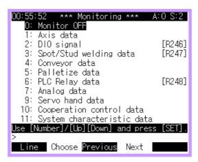
(2) Press the [SET] key after selecting desired item by using the [Number] key or the arrow key.
