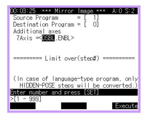
If 'Limit over(step#)' indicates 'Completion,' it means review is over. If 'Steps Exceeding Limit' indicates '=>,' it means there are more steps exceeding limit.
