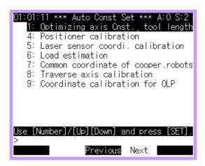
(2) Use the [Arrow] keys to move to the item to select and press the [SET] key or press the number of the item to choose using the [Number] key and press the [SET] key to enter the sub menu.
