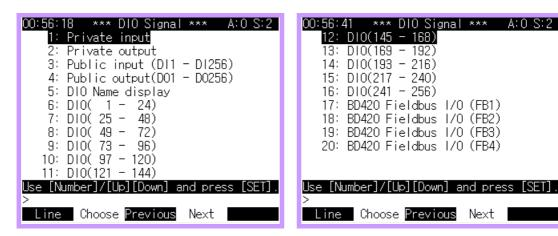
(2) Press the [SET] key after selecting desired item by using with the [Number] key or arrow key.
