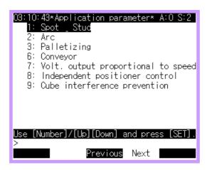
(2) Use the [Arrow] keys to move the cursor to the item to select and press the [SET] key. Or you can enter the number of the item to select and press the [SET] key to move to the sub menu.
