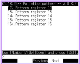
(2) Use the [Arrow] keys to move the cursor to the item to select and press the [SET] key. Or you can enter the number of the item to select and press the [SET] key to move to the sub menu.
