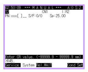
(3) Input value of Conveyor Register with the [Number] key and then prerss the [SET] key.
