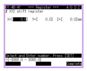
(2) Input data in X,Y,Z and press [SET]. To store changed setup, press  $\lceil$ [PF5]: Complete $\rfloor$  . If [ESC] is pressed, changed data will not be stored.
