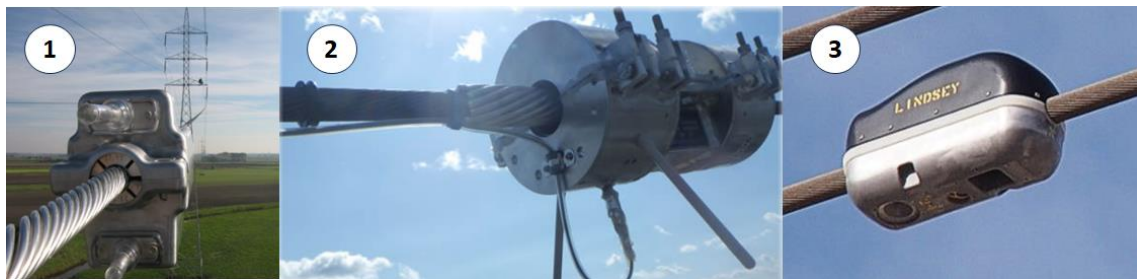
Figure 3 – Models of Dynamic Line Rating (DLR) (1: Ampacimon; 2: DLR Sensor Sumitomo; e 3: Lindsey TLM Conductor Monitor)
