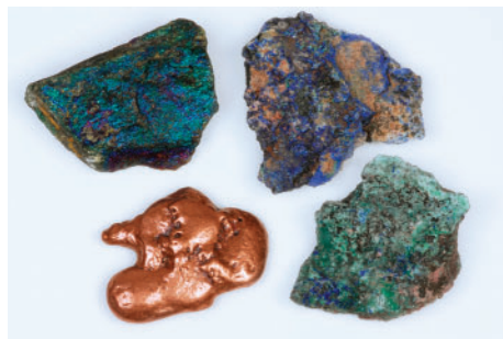
Figure 2 Clockwise from lower left: native copper, bornite, azurite, and a mixture of malachite and azurite. Only native copper contains copper atoms. The other minerals contain either \text{Cu}^+ or \text{Cu}^{2+} ions.
