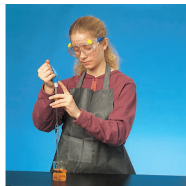
Figure 6 Release the bulb slowly. Pressing down with your thumb placed across the top of the bulb maintains a good seal. Setting the pipette tip on the bottom slows the rise or fall of the liquid.
