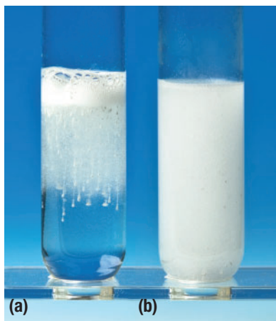
Figure 3 Powdered magnesium metal reacts with (a) hydrochloric acid and with (b) ethanoic acid. The foam in test tube (a) indicates that oxygen is produced much more rapidly than in test tube (b).
