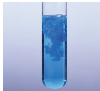
Figure 4 Combining solutions of sodium hydroxide and copper(II) sulfate produces a jellylike precipitate of copper(II) hydroxide.
