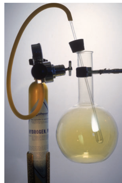
Figure 4 Colourless hydrogen gas from the tube reacts with yellow chlorine gas in the cylinder to produce toxic hydrogen chloride gas.
