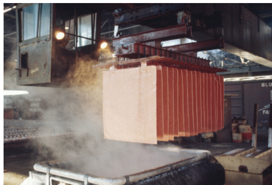
Figure 1 Refining metals, such as these sheets of pure copper, produces toxic metal ions. These ions must be removed before the wastewater can be discharged.
