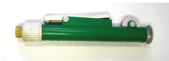
Figure 8 Pipette pumps have a small roller that can be turned to draw liquid in or to let liquid out of the pipette.
