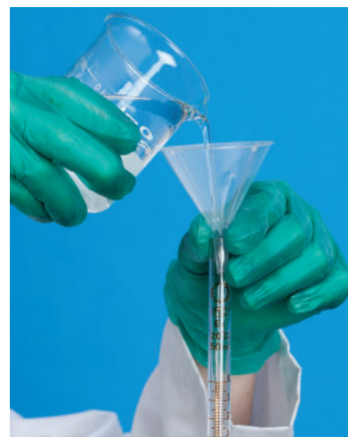
Figure 6 A tight-fitting funnel prevents the titrant from draining into the flask. Raise the funnel slightly if necessary.
