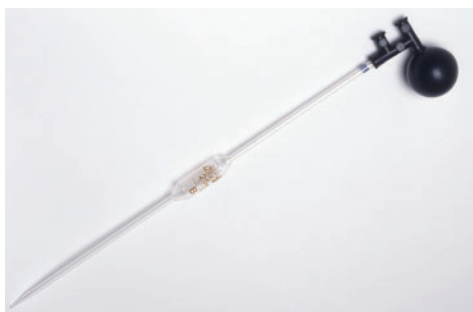
Figure 7 A dispensing pipette bulb uses a small valve in the side stem to control the flow of liquid in a pipette.
