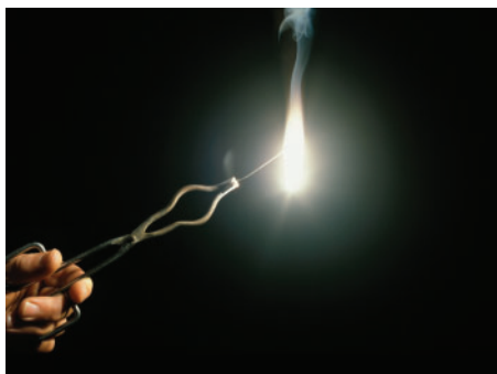
Figure 2 Burning magnesium emits a light that is bright enough to damage your eyes. You should only look at the flame through a UV safety shield.
