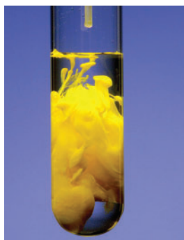
Figure 1 Lead and iodide ions combine to form a precipitate of lead(II) iodide, \text{PbI}_2(\text{s}) .
