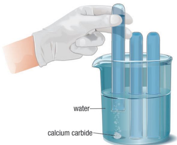
Figure 2 Collect the gas produced when calcium carbide reacts with water.
