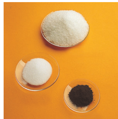
Figure 5 Samples of 1 mol each of sucrose, sodium chloride, and carbon. All three samples contain the same number of entities.
