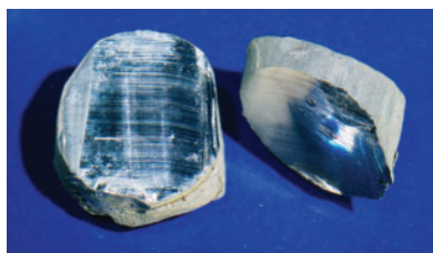
Figure 7 A cylinder of sodium has just been cut, exposing the shiny metal. Within seconds, a layer of dull sodium oxide will cover this shiny surface.
