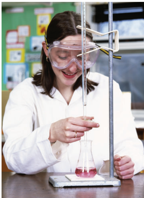
Figure 1 Run the titrant into the sample slowly as you approach the endpoint.
