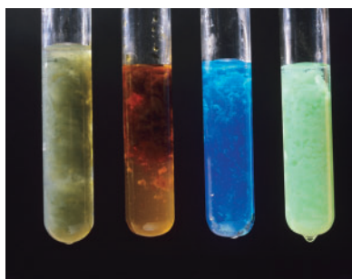
Figure 2 Precipitates form when a solution of sodium hydroxide is added to solutions of metal compounds.
