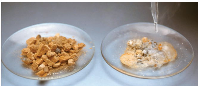
Figure 1 Calcium carbide reacts with water. Ethyne is less dense than air. This means that ethyne rises quickly when it is released in the air, just like a helium-filled balloon.
