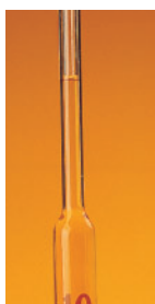
Figure 9 To allow the liquid to drop slowly to the calibration line, it is necessary for your finger and the pipette top to be dry. Also keep the tip on the bottom to slow down the flow.
