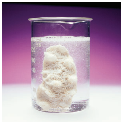
Figure 4 Coral contains mostly calcium carbonate. This compound neutralizes sulfuric acid. Bubbles of carbon dioxide appear as the reaction proceeds.
