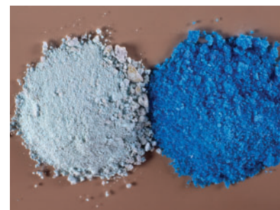
Figure 4 Hydrated copper(II) sulfate is a distinctive blue colour. When the same copper compound has no water in its structure, it is white.
