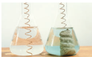
Figure 1 The reaction of copper wire in a solution of silver nitrate. The blue colour of the solution is evidence that \text{Cu}^{2+}(\text{aq}) ions are produced.
