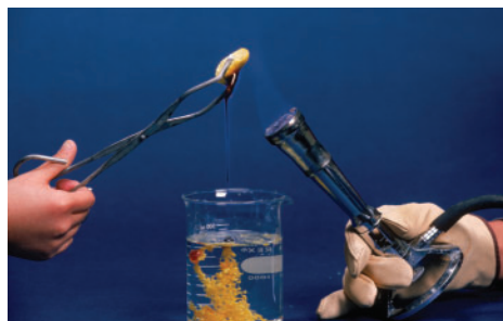
Figure 2 Sulfur is a solid, yellow non-metal that burns with a blue flame to produce colourless sulfur dioxide gas. Liquid sulfur is dripping into the beaker and solidifying.
