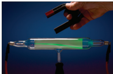
Figure 3 J.J. Thomson used a device known as a cathode ray tube to perform his experiments.
