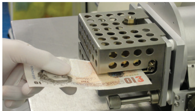
Figure 2 Thermal desorption apparatus vaporizing organic compounds off a banknote
