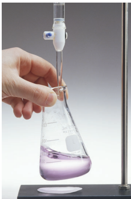
Figure 12 Near the endpoint, continuous gentle swirling of the solution is particularly important.
