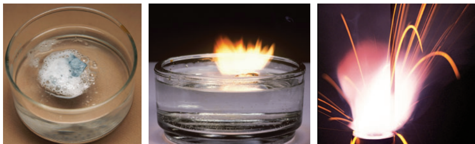
Figure 2 The alkali metals (lithium, sodium, and potassium) are all reactive when mixed with water.
