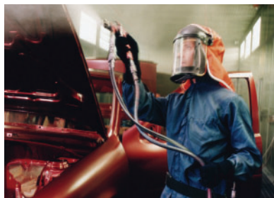
Figure 7 The VOCs from automotive paint can be toxic. An airtight mask and respirator prevent this worker from inhaling toxic fumes.
