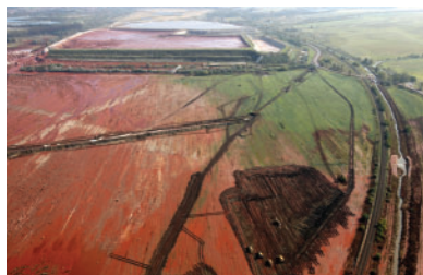
Figure 8 The red mud that flowed out of the holding pond in Hungary had a very high pH and contained potentially dangerous metal ions.
