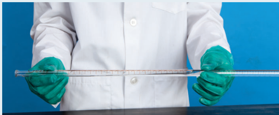
Figure 7 Roll the burette in your fingers to wet the inner surface with titrant.
