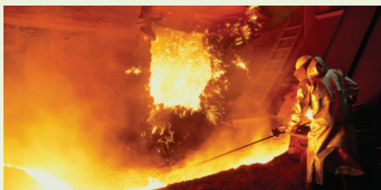
Figure 9 A steel foundry heats coke (carbon) and other ingredients with iron ore (mostly \text{Fe}_2\text{O}_3 ) to convert it into molten iron.
