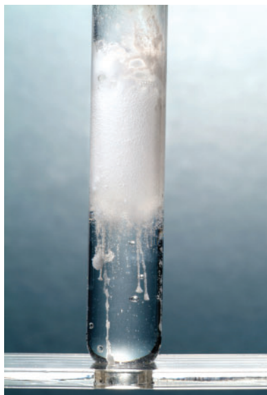
Figure 7 The reaction of magnesium carbonate and hydrochloric acid results in the production of a gas.
