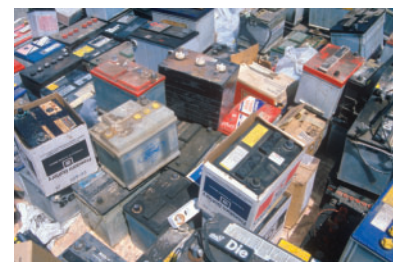
Figure 1 Old car batteries contain lead, a toxic metal, and corrosive sulfuric acid.
