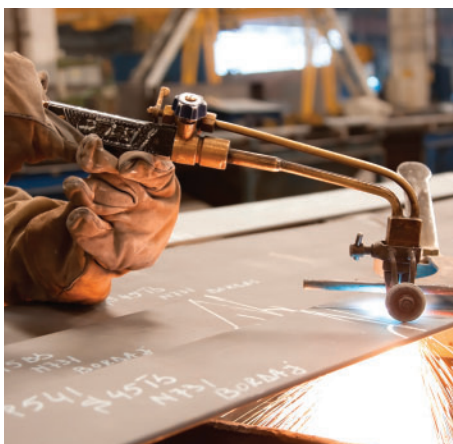
Figure 3 The two pipes in an oxyacetylene torch carry oxygen and the fuel from storage tanks to the nozzle.
