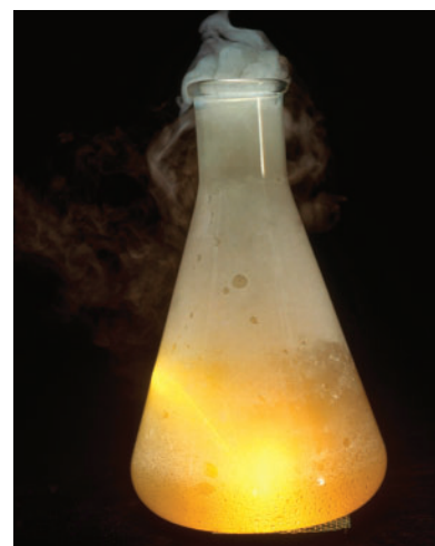
Figure 4 Sodium metal and chlorine gas react violently to form sodium chloride (table salt).
