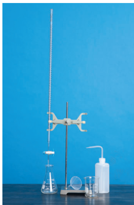
Figure 11 A burette should be rinsed with water and then with the titrant before use.
