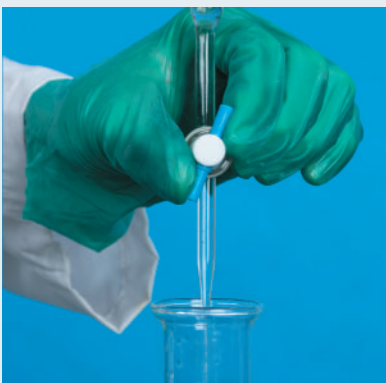
Figure 11 Allow the titrant to flow into the flask. Prepare to reduce the flow as you approach the endpoint.
