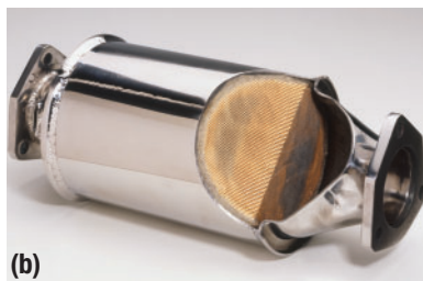
Figure 6 (a) The catalytic converter, situated between the engine and the tailpipe, is part of a car's emission control system. (b) The ceramic matrix inside is covered with beads of platinum, palladium, and rhodium.
