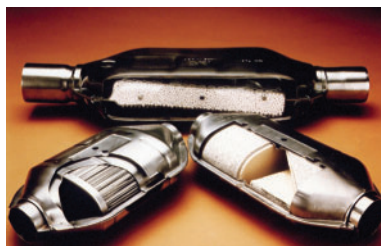
Figure 2 A catalytic converter is part of the exhaust system in an automobile.
