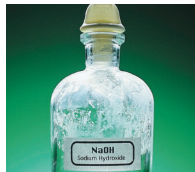
Figure 14 Sodium hydroxide reacts with carbon dioxide to form solid sodium carbonate. If the mouth and glass stopper of this bottle are not cleaned regularly, sodium carbonate can glue the stopper to the bottle, making it almost impossible to open.
