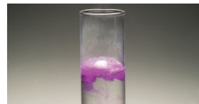
Figure 6 The reaction of sodium metal (small ball in the centre) with water containing phenolphthalein indicator. The magenta colour of the indicator shows that hydroxide ions are being produced.
