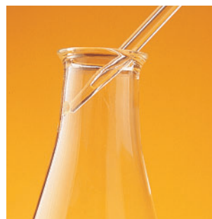
Figure 10 A vertical volumetric pipette is drained by gravity and then the tip is placed against the inside wall of the container. A small volume is expected to remain in the tip.
