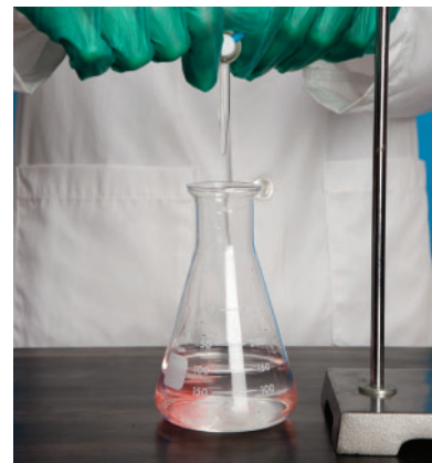
Figure 13 The endpoint has been reached when a single drop of titrant results in a colour change that does not fade when the mixture is swirled.
