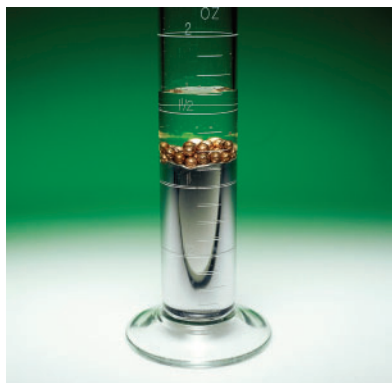
Figure 1 This graduated cylinder contains mercury (bottom), copper beads (middle), and salt water (top).
