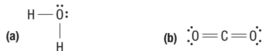
Figure 6 Lewis structures of (a) water and (b) carbon dioxide show how different elements can share valence electrons to form stable molecules.
