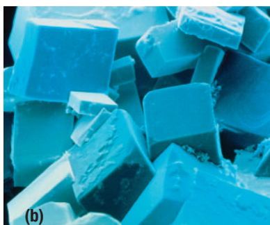
Figure 5 (a) Sodium chloride, \text{NaCl}(s) , is made up of equal numbers of positive and negative ions. (b) Sodium chloride crystals are cubic in shape, as this image, taken with a scanning electron microscope, shows.
