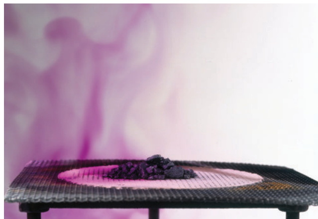
Figure 4 Iodine is a violet-black solid that gives off corrosive iodine vapour when heated. Iodine was originally extracted from seaweed.
