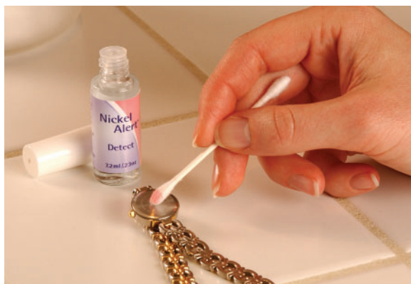
Figure 2 A qualitative test shows the presence of nickel ions in the casing of a watch.
