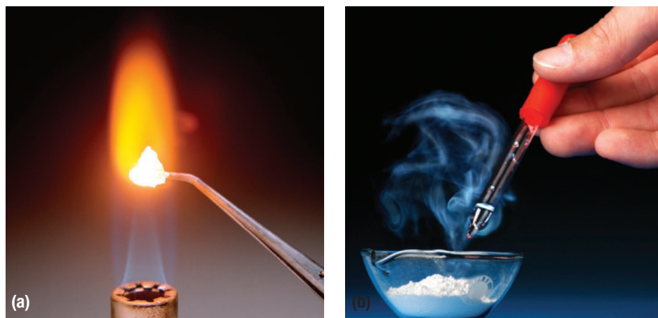
Figure 9 (a) Calcium burns to produce calcium oxide, \text{CaO}(\text{s}) . (b) Adding water to calcium oxide produces calcium hydroxide and so much energy that steam rises from the mixture.
