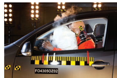
Figure 4 An automobile airbag is designed to inflate in a fraction of a second.
