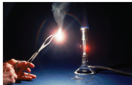
Figure 3 Magnesium metal burns with a white-hot flame to produce magnesium oxide, a white powder.
