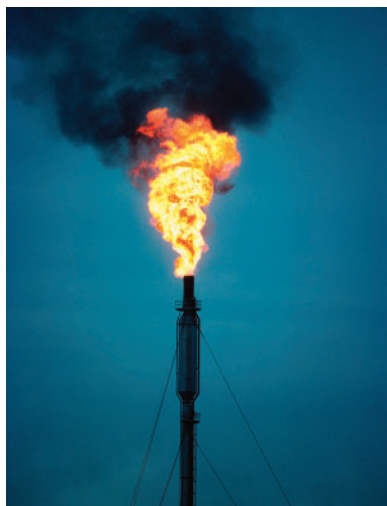
Figure 4 The combustion of excess hydrocarbons at an oil refinery produces yellow flames and soot. These are both evidence of incomplete combustion.
