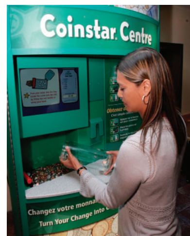
Figure 3 Coin-counting machines stack coins and use height or mass to determine how much to pay out.
