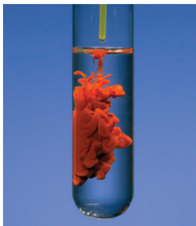
Figure 2 Adding yellow potassium chromate solution to colourless silver nitrate solution produces solid red silver chromate.
