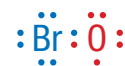
Figure 4 Lewis structure of a bromine monoxide molecule. This molecule is reactive because of the single electron on the oxygen atom.
