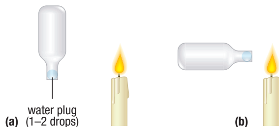
Figure 4 Keep the bulb pointing down until you are ready to push the gases into the flame.
