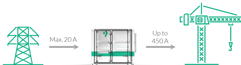
Connection between the utility mains, Enertainer and the load.
