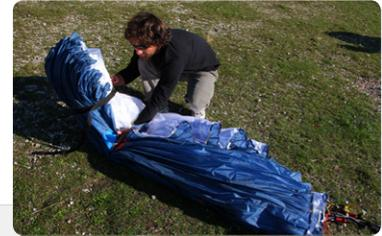
**Step 6.** Fold the wing with 3 or 4 folds whilst being careful not to crush the LE.
