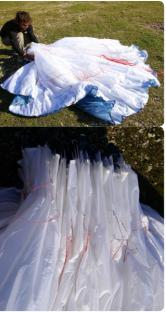
**Step 3.** Lay wing on its side and Strap LE...Note the glider is NOT folded in half; it is folded with a complete concertina from tip to tip. It is really important to not stress the middle cell or bend the plastic too tightly.
