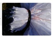
**Step 4.** Group together the middle/trailing edge of the wing by sorting the folds near the B, C and D tabs.
