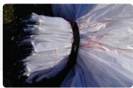
**Step 4.** Group together the middle/trailing edge of the wing by sorting the folds near the B, C and D tabs.
